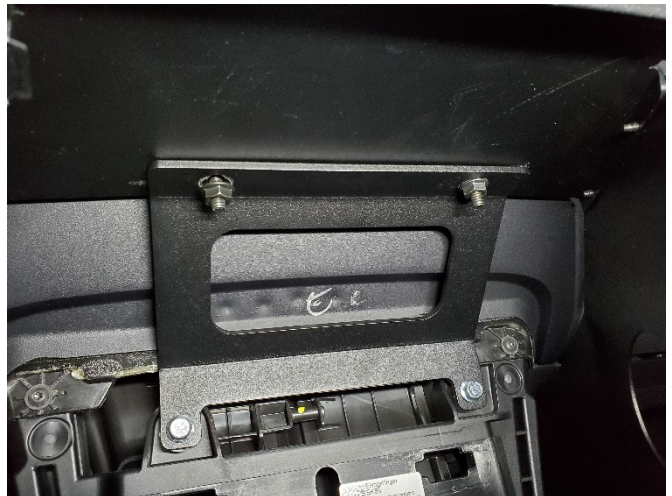
Attach top of console to upper mounting bracket with (2) 1/4" x 3/4" Carriage bolts and serrated nuts.
