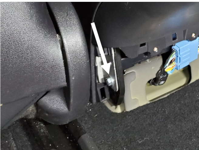
Remove (2) 10mm head bolts from rear, sides of console.
