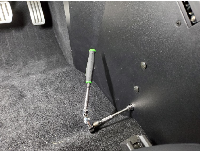
Tighten bolt through access hole in side of console. Install 1" dome plugs to cover access hole in console. (Repeat for other side)
