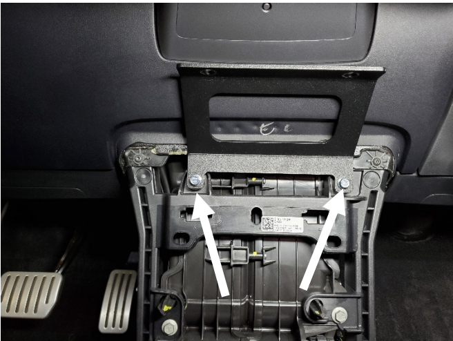
Attach upper mounting bracket to dash using 3/8" plastic spacers and M6 bolts.
