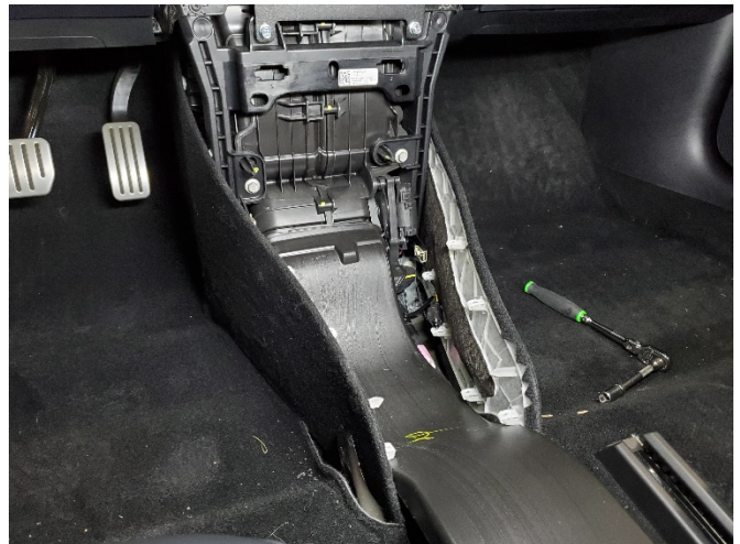
Reattach factory carpeted trim. Reattach ductwork to center output on dash.
