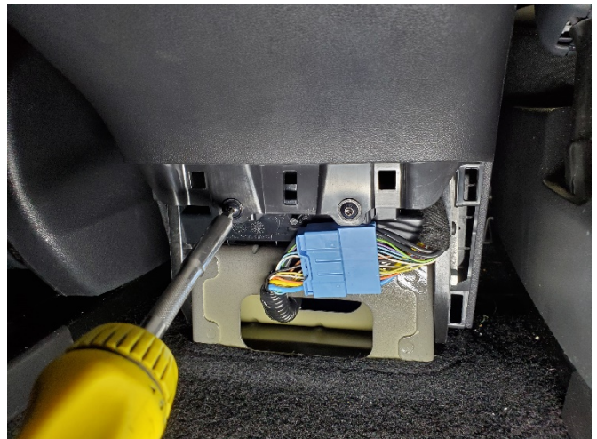
Remove trim cover from rear of center console housing. Unplug connector, and remove (2) T-20 Torx head screws.
