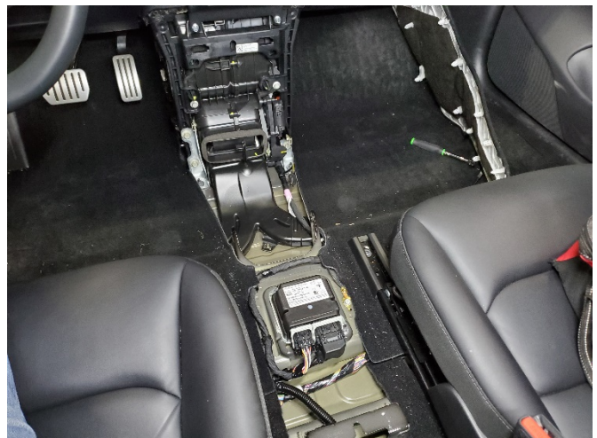
Unplug harnesses as needed and remove center console from vehicle.
