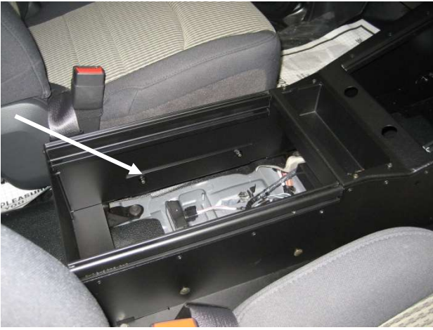
Place main console housing onto floor mount platform and fasten together with 1/4 x 1/2 carriage bolts and serrated nuts.
