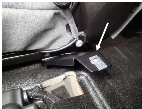
Optional CM006059 Passenger side rear bracket with GSM33001 (1/4 x 3/4 screws) and GSM31005 (1/4 flat washers) (Included in C-B66 kit)
