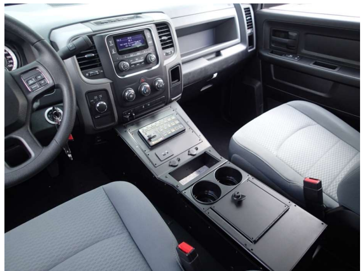
Completed C-VS-0814-RAM-2 console installation
