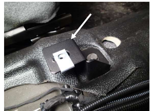
Optional CM006056 Driver side forward bracket with GSM33745 (M8 x 35mm bolt) and GSM31007 (3/8 flat washer) (Included in C-B66 kit) Shown with GSM30106 (5/16 clip nut)
