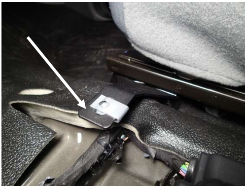
Optional CM006058 Passenger side forward bracket with GSM33119 (10/32 x 3/4 screws) and GSM31003 (#10 flat washers) (Included in C-B66 kit)
