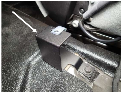
Optional CM006057 driver side rear bracket with GSM33745 (M8 x 35mm bolt) and GSM31007 (3/8 flat washer) (Included in C-B66 kit) Shown with GSM30106 (5/16 clip nut)
