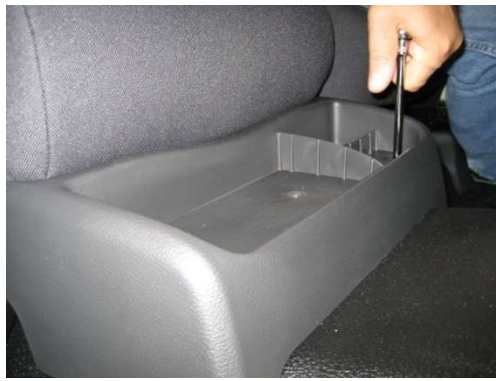
Remove center seat front accessory pocket. (If applicable) Special Service truck will not have center seat (Phillips Screwdriver)
