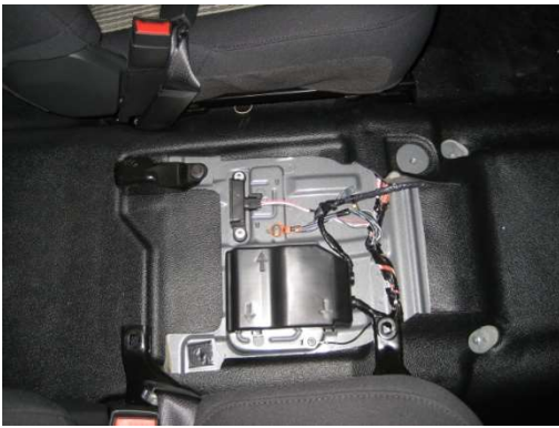
Remove center seat section from floor mount brackets. (13 mm socket) Do not remove OEM seat brackets NOTE: The OEM air duct will work in original location. If air duct is not used, installer must plug duct outlet. Some vehicles will not have air duct.
