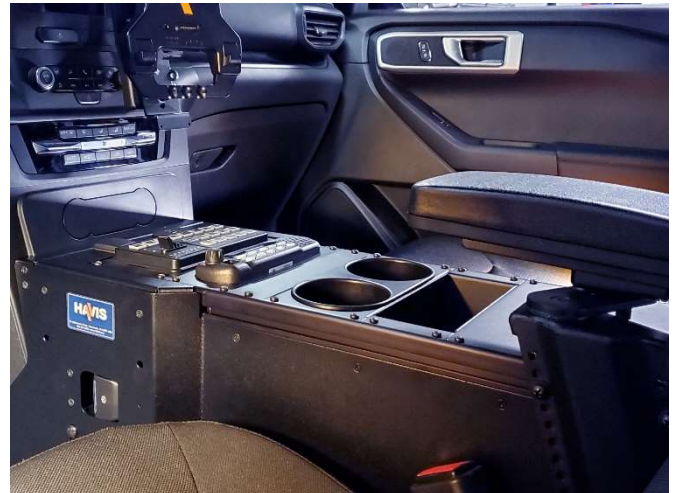
Relocate OEM 12 volt socket and USB into console. Wire and install equipment as needed. Installation is now complete.
