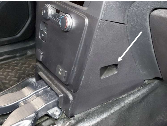
Remove fasteners on sides of lower trim. (7mm)
