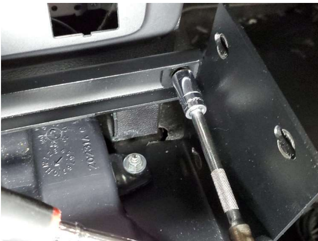
Attach front and rear forward cross supports using (4) 1/4" x 1/2" carriage bolts and nuts.
