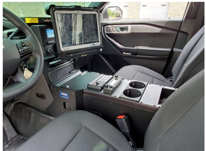
Views showing optional C-CUP-1001 cup holder, C-PM-124 printer mount and C-DMM-3015 dash mount with Tablet docking station.
