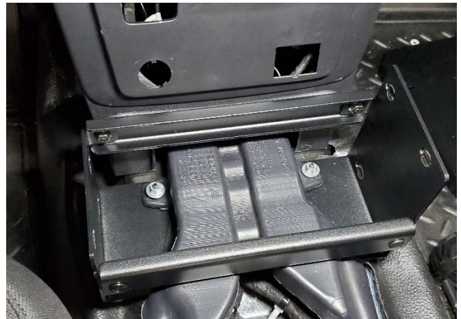
Tighten OEM nuts. (10 mm socket)
