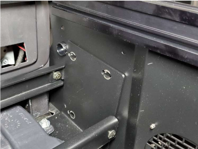
Attach housing to front brackets with 1/4" x 3/4" carriage bolts and serrated nuts.
