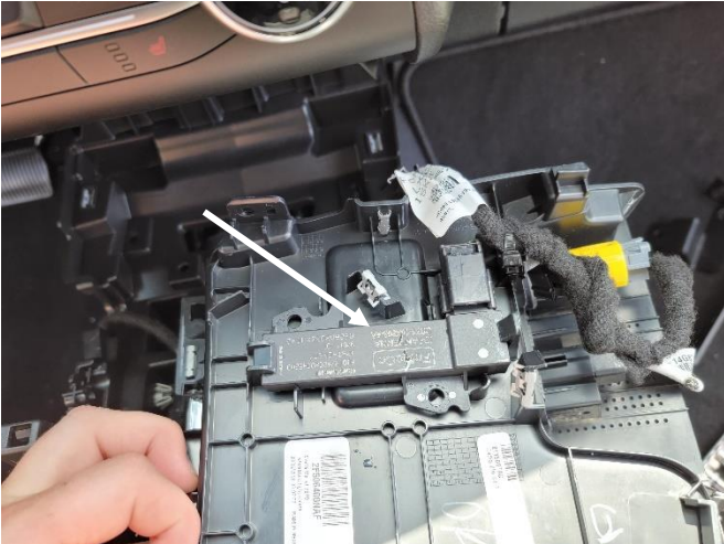
Unplug USB, 12v socket, and key sense module. Remove key sense module.
