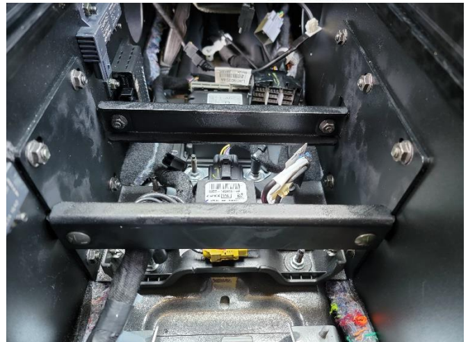
Attach cross braces onto floor mounting brackets with 1/4" x 1/2" Carriage bolts and nuts.
