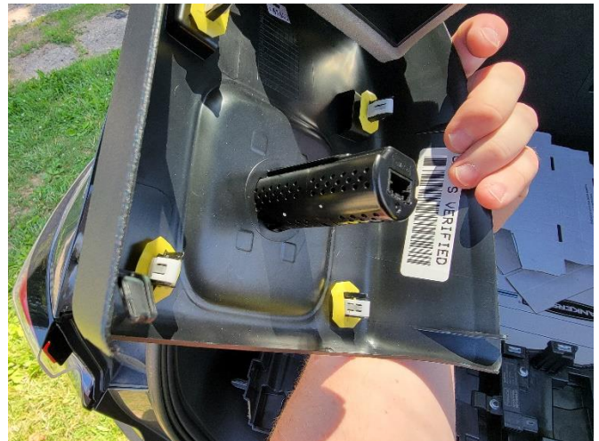
Remove OEM USB plug from rear console plate.
