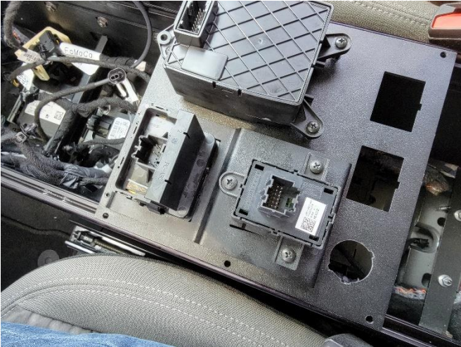
Attach Mode plate to shifter plate using flat head screws.
