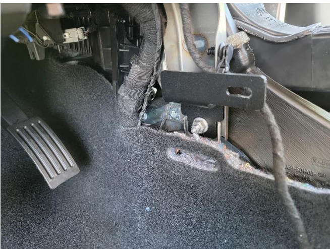
Using bolt removed at the beginning of the install, add Driver side forward mounting bracket.
