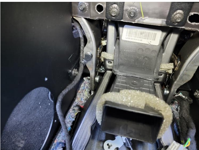
Using supplied foam block, install into center vent tube. Be sure to fully block off vent. Add duct tape if desired to ensure a good seal.
