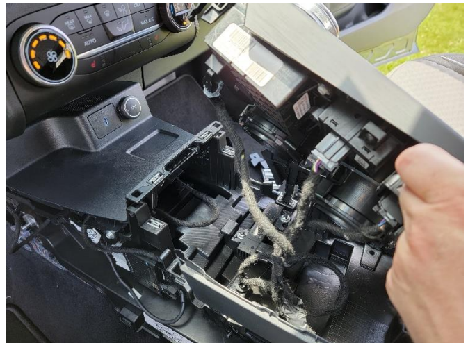
Unplug all harnesses from OEM modules.
