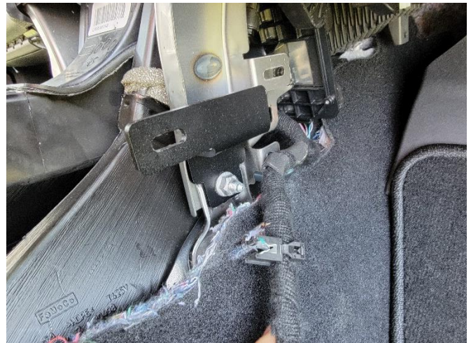
Install Passenger side forward mounting bracket.
