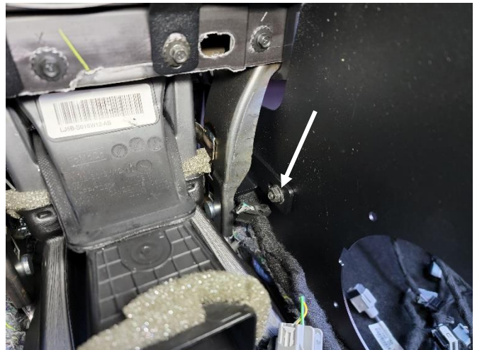
Attach to front, floor mounting brackets using 1/4" x 3/4" carriage bolts and serrated nuts.
