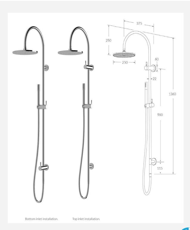
Able to be installed top or bottom inlet. No additional component will be required.
