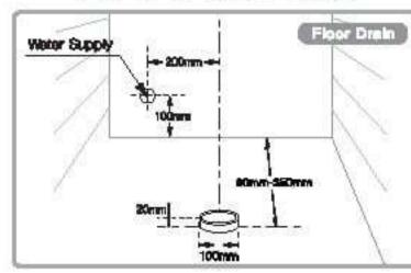
200mm-350mm - Ceramic Pan (S-Trap) 80mm-200mm - Acrylic Pan (S-Trap)
