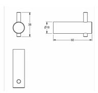
Hook for wall mounting, stainless steel, surface satin finished, 17 mm pipe diameter, drilled hole on bottom for fixation, incl. stainless steel screws and dowels.
