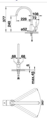
Note: Measurements are within 2 - 3mm of factory tolerance. It is advisable to check dimensions of physical product when measuring for installations and before doing any cut outs. \*Due to continual product development the information provided is not final and may be subject to change.
