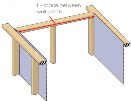
When following **Detail 1**, sheet bathroom walls except for wall with Shadowline Diffuser. For **Detail 2**, sheet all walls Measure the space between the walls where the Shadowline is to be installed. The total Shadowline Diffuser length must be 2 - 5mm less than this to provide some tolerance for fitting.
