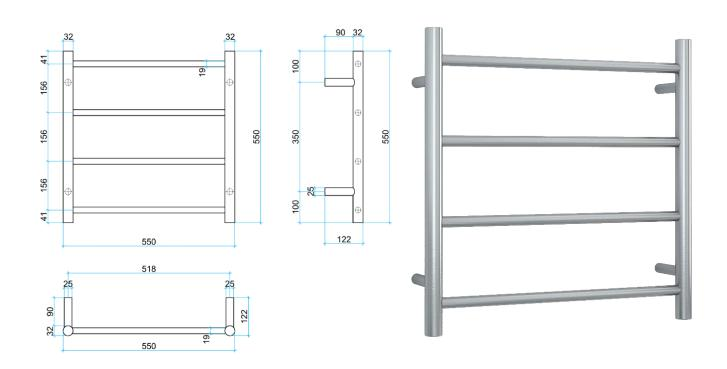
This rail has Multiflex wiring which means that there is a connection point on both the left and right hand side of the rail and the lead can be connected to either side. Being a dry electric element rail, this can be mounted either way up meaning the wiring can be from any of the four mounting points.
