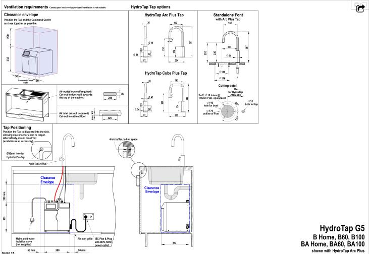
SAGLE 1:3 ALL DIMENSIONS IN MM UNLESS OTHERWISE SPECIFIED. INSTALLATION DIAGRAMS ARE FOR ILLUSTRATIVE PURPOSES ONLY. HOSES ARE NOT SHOWN TO SCALE AND CANNOT BE LENGTHENED
