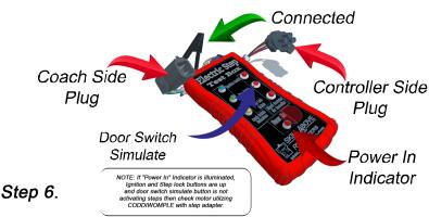
With Coach and Controller side plugs as well as green chassis ground cable connected the door switch latching push button will simulate the coach door switch signal to the controller.
