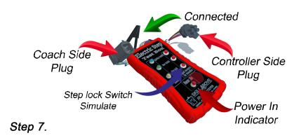
With Coach and Controller side plugs as well as green chassis ground cable connected the Step lock latching push button will simulate the coach Step lock switch signal to the controller.
