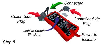
With Coach and Controller side plugs as well as green chassis ground cable connected the ignition latching push button will simulate the coach ignition switch signal to the controller.
