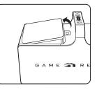
2 Add water to fill-line indicated on label within the reservoir. DO NOT OVERFILL. Add ice to top of reservoir.
