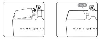
Place the Control Unit in the location where you plan to use it. The Control Unit should only be used in the upright orientation as shown. The Control Unit will leak if placed on its side.
