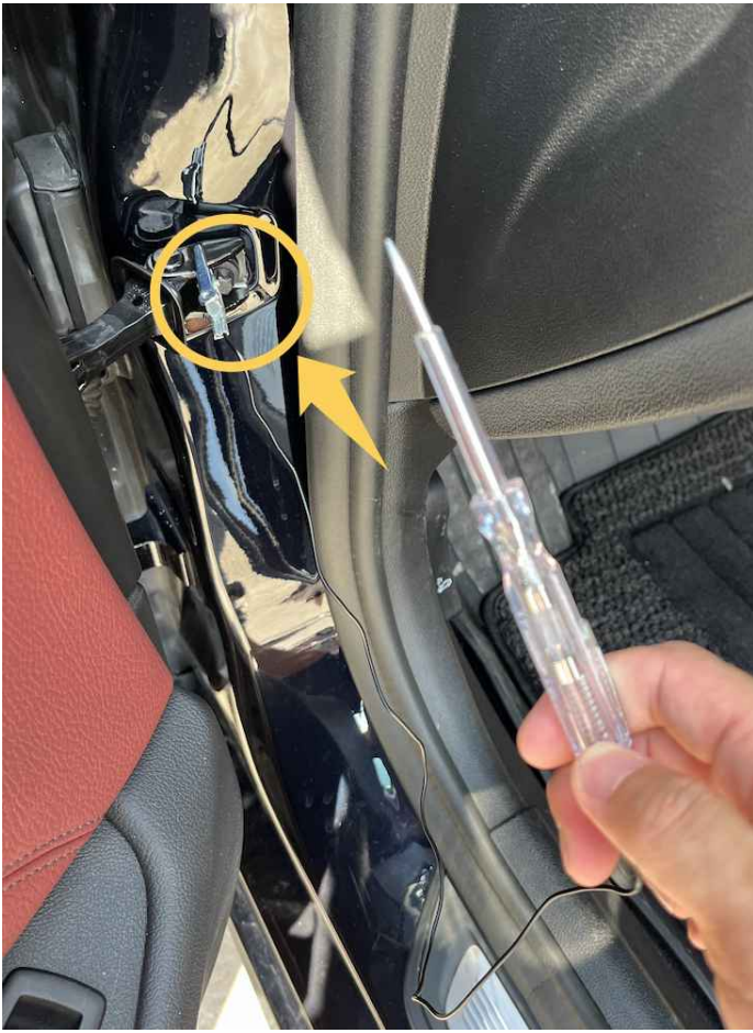
Connect circuit tester to the metal (ground)
