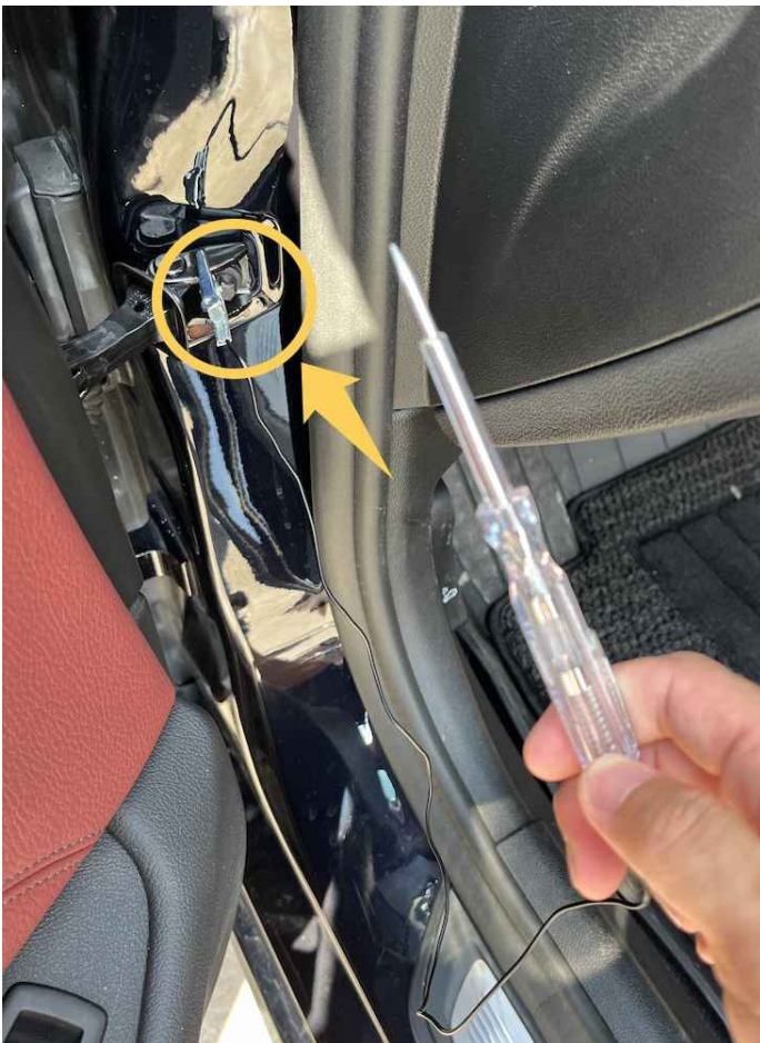
Connect circuit tester to the metal (ground)
