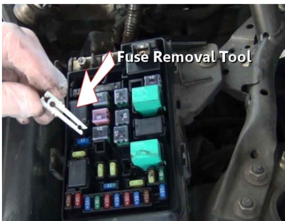
There may be a fuse removal tool in the fuse box next to the engine.
