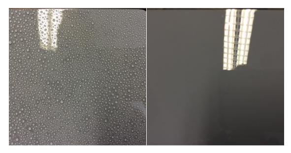
**Picture on the left:** the activator is visibly beading on the surface. Beading indicates the activator is not yet ready for use. Applying the silver solutions over the beading activator will result in a spotty looking chrome effect.
