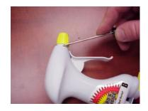
Make a note as to which way round this red rubber insert goes in. This will need to be cleaned as the silver forms around the red rubber and the white surround also.
