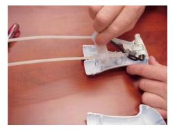
Remove trigger / piston drive yoke and pump assembly from sprayer body.
