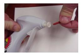
Separate the sprayer body. Disengage latch located on the bottom of body between bottle locks.
