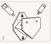
1. Place the lamp socket on the wall and secure it with two of the included screws
