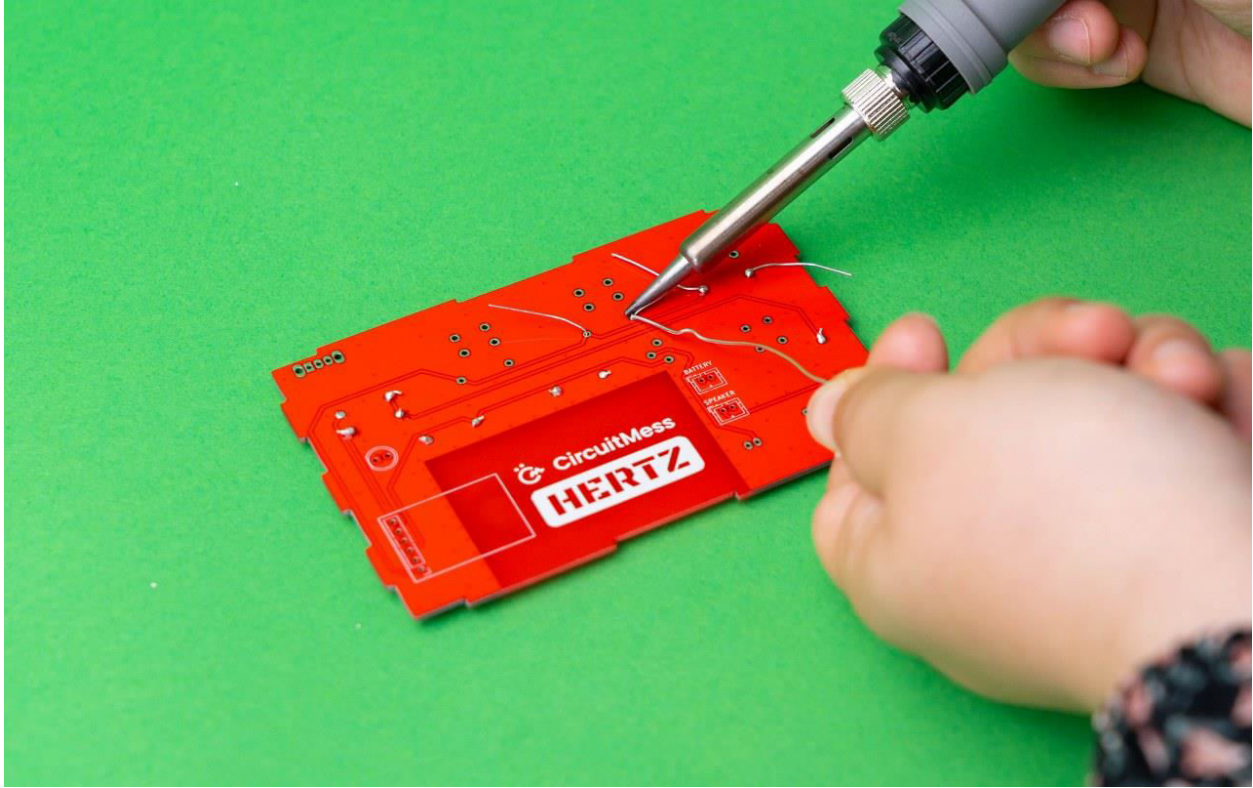
After you have soldered all three resistors, you can cut its legs.
