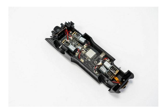
It's time to fasten the motors to the chassis.
