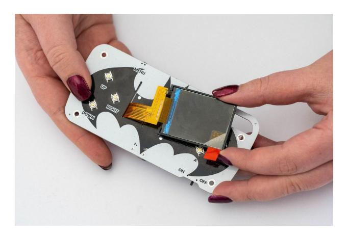
After pulling the ribbon through, the back of the PCB should look like this.
