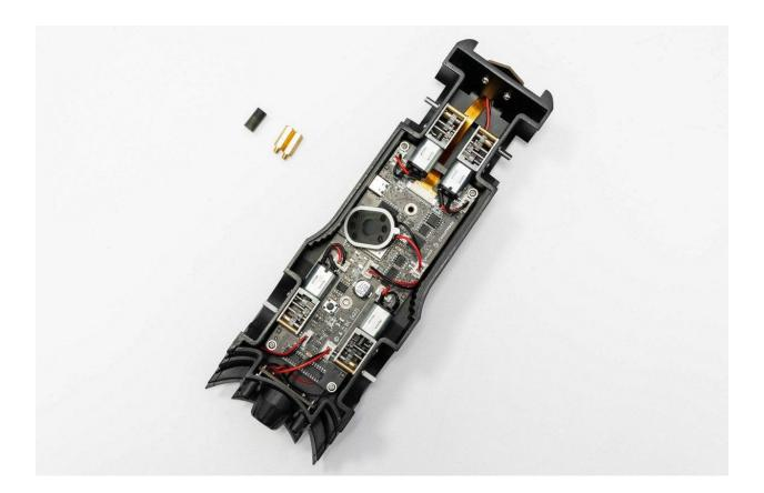
The golden spacers go into the holes in the middle of the PCB.
