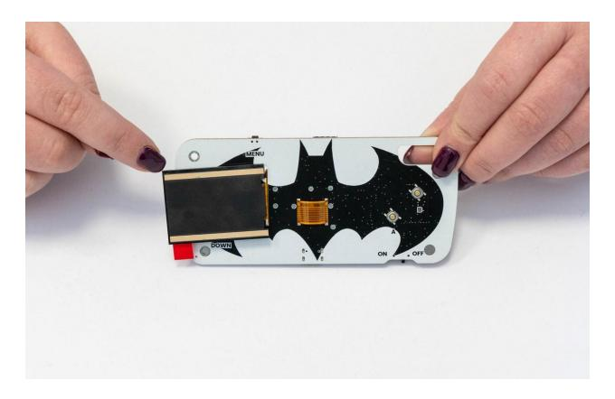
You must remove the stickers and stick the display to the PCB.
