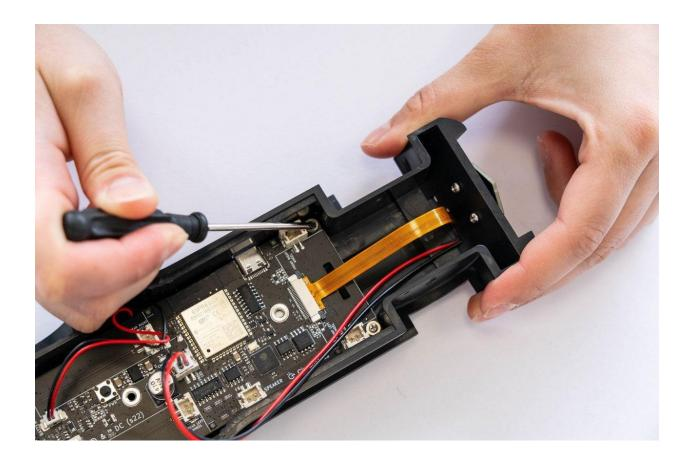
If all the wires and ribbons are connected and the PCB is tightened, you may proceed.
