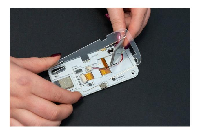
You'll need to place the wires under the casing so they don't get in your way, and then press the battery into its place.
