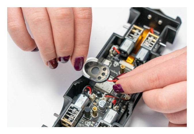
Make sure the casing is on the right side and attach the speaker to it.
