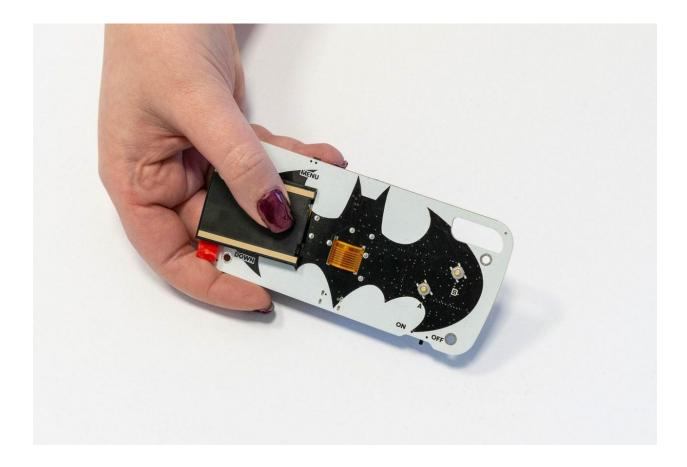
Finally, connect the ribbon to the PCB.
