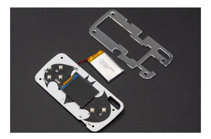
Check the cuts on the acrylic casing before proceeding to ensure proper placement on the PCB.
