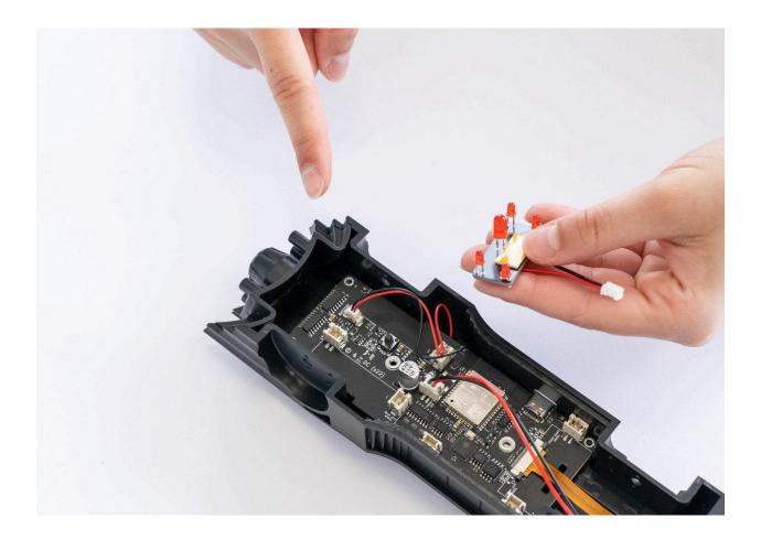
Connect the fire board to the "LED Fire" port.
