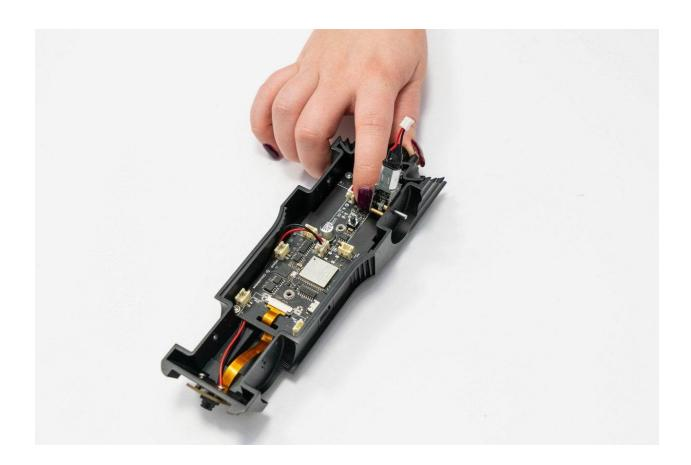
Connect the motor wire to the port below it:
