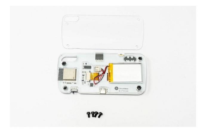
Place the casing on top of the Batcontroller first:
