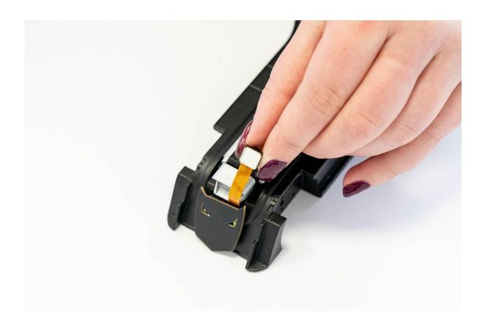
Stick the camera between the "eyes" of the Batmobile in the middle of the headboard.
