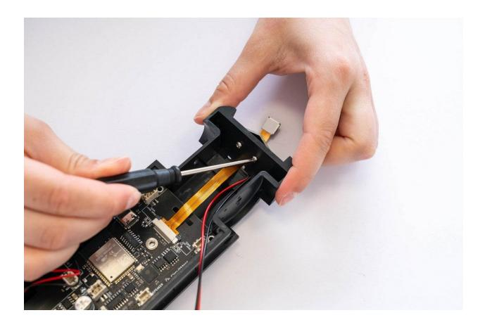
After you've tightened the headboard, you can attach the camera to it.
