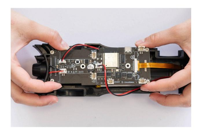
Put it back down slowly to make sure the screws fit inside the chassis.
