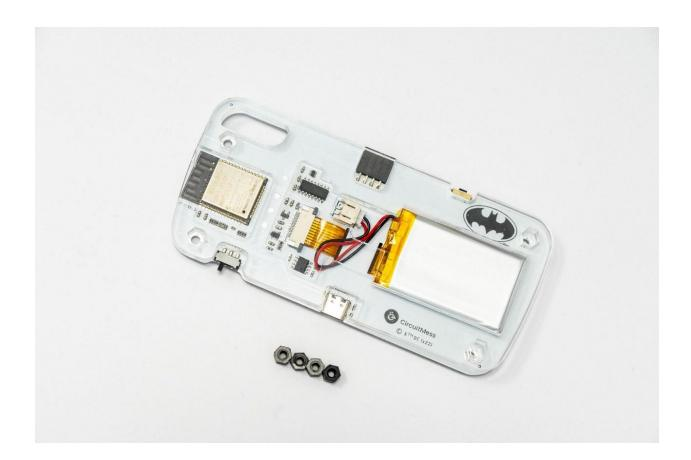
You must insert one black spacer into each of the four holes.
