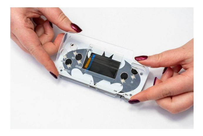
Place one of the button caps at each of the six dots indicating where the pushbuttons should be (left, right, up, down, A, and B).
