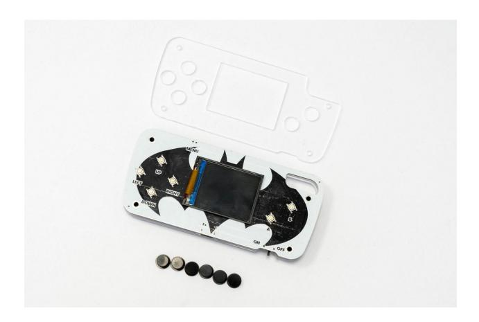
To begin, we must place the casing on top of the Batcontroller:
