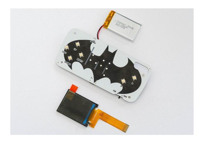
Make sure the display is on the correct side and that the ribbon is pulled through the correct hole.
