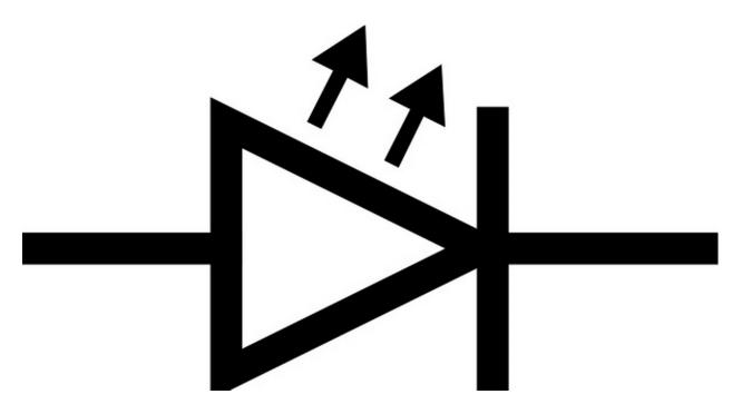
Watch out - LEDs are polarized!
