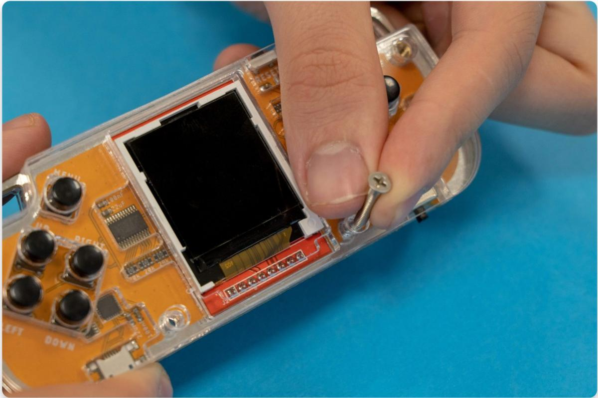
Take the spacer and place it on top of the bolt from the back (mostly white side of the board). Tighten the bolt and the spacer using the screwdriver. Repeat the same process for the other hole.
