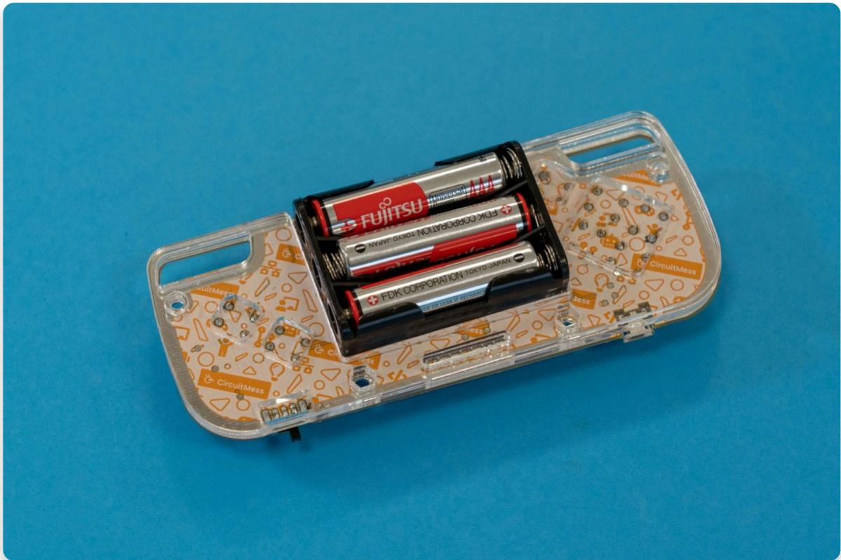
After you layered the back casings, take the first layer of the front casing and place it at the front while holding the ones in the back.
