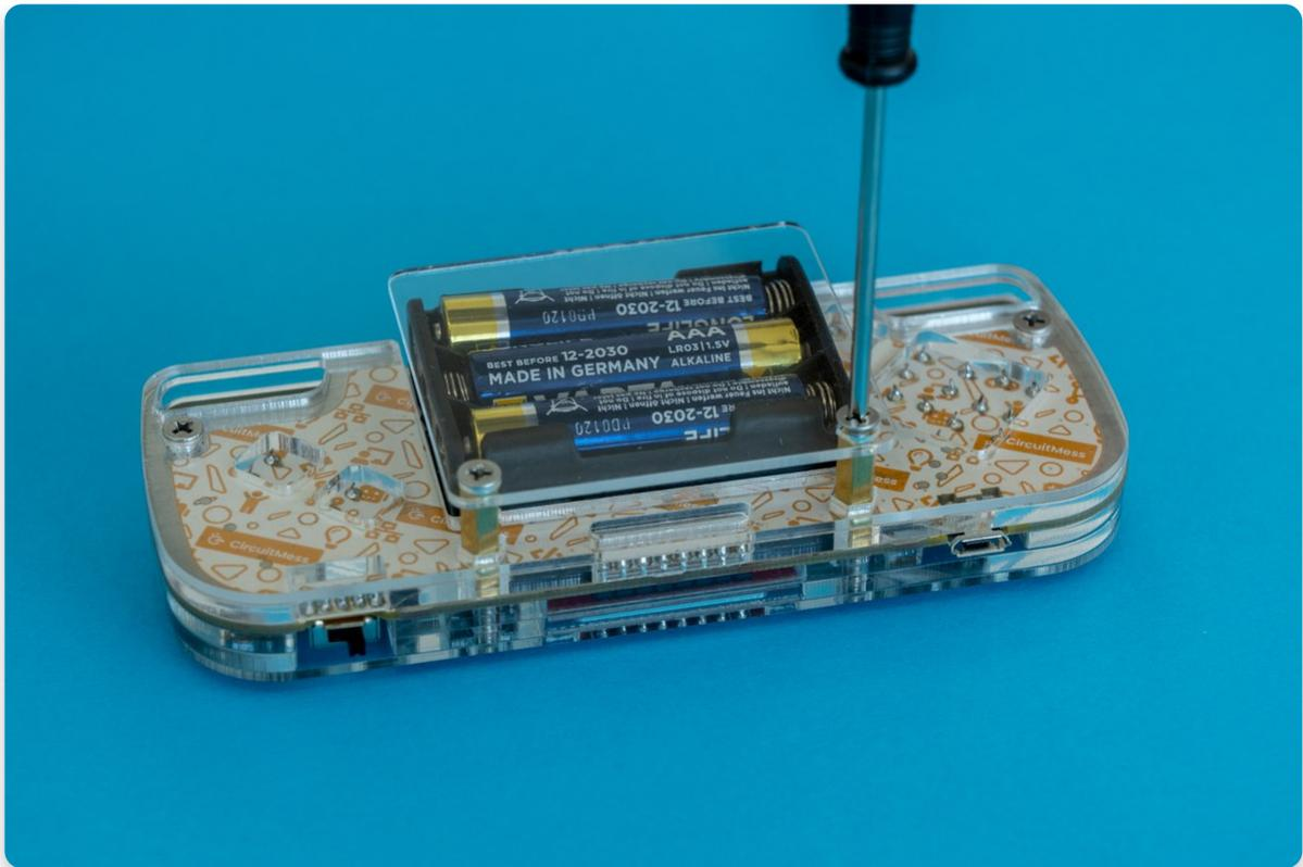
Tightening the bolts on the battery cover
