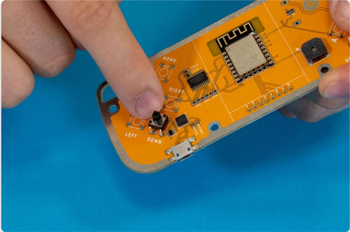
Take one of the mechanical button parts and put it through the holes. There are a total of **seven button placement locations**, each with four little holes, that mark the following buttons: **MENU, UP, LEFT, DOWN, RIGHT, A, and B.**
