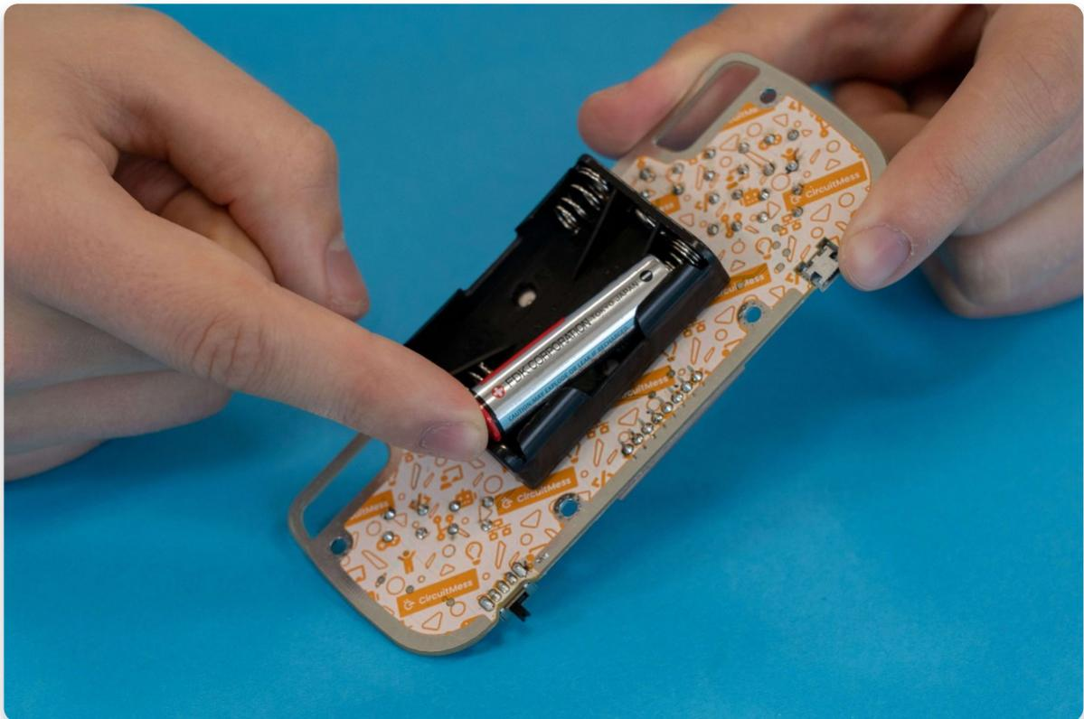
**Repeat the same process for the other outer battery slot.**
