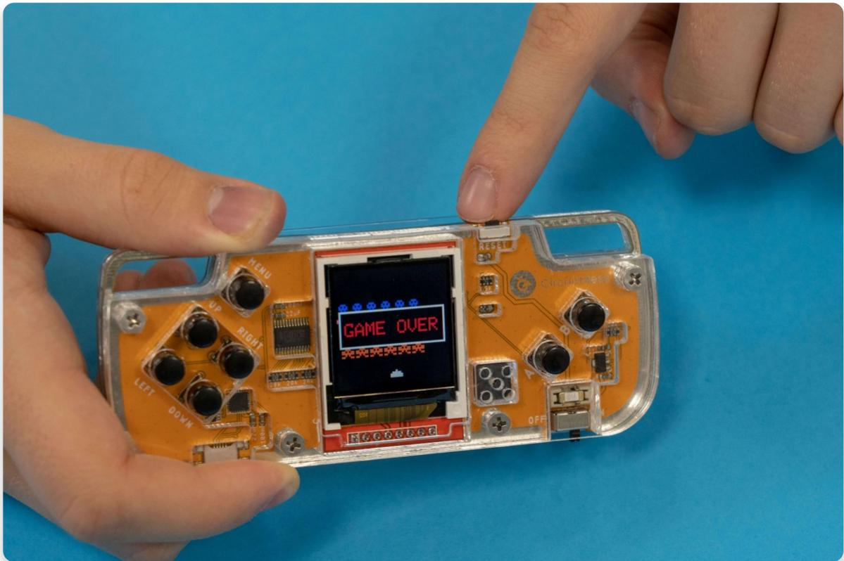
There is also a small blue light underneath the screen that should be blinking while the console is on. You probably won't see it from all these casings, but if you do, don't be surprised - it's an indicator that your console is working.
