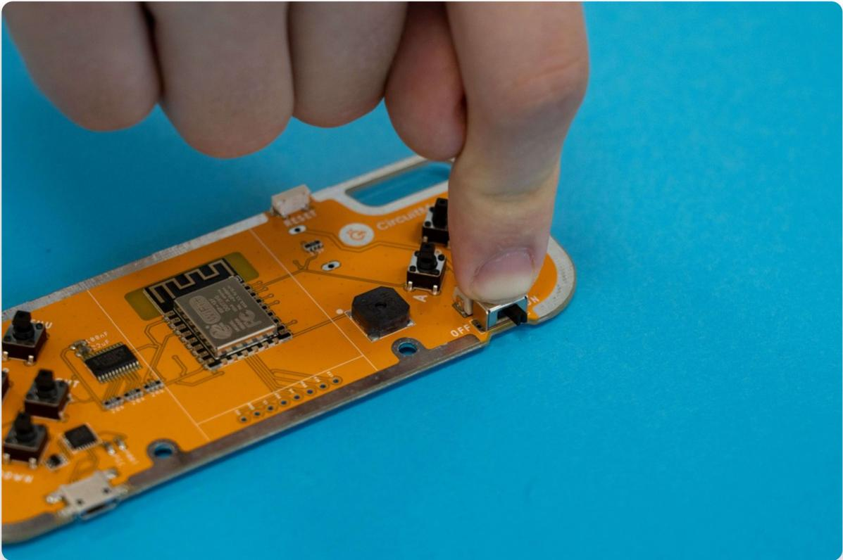
Make sure all the pins go through all the way so that the component is as close to the board as possible.
