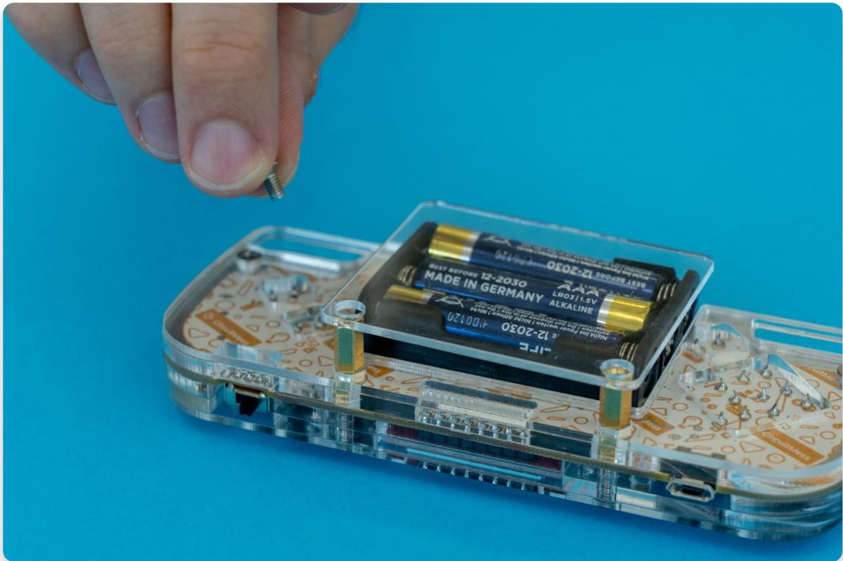
Putting the plastic cover on top of the batteries
