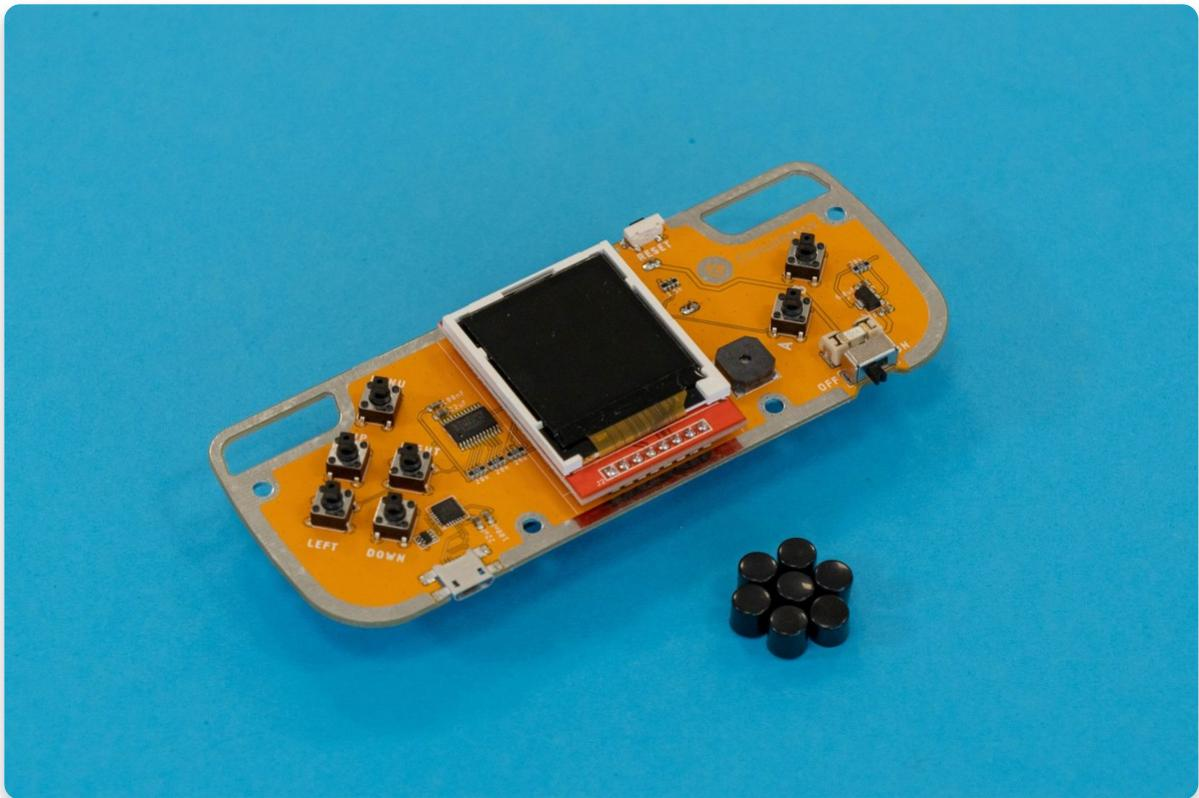
The process of putting them on is nothing too complicated. Just take a button cap and put it on top of the button. Press hard so the button cap properly clicks on. If the button cap remains on after you release it, and the button can still be clicked, you've put the cap on properly!
