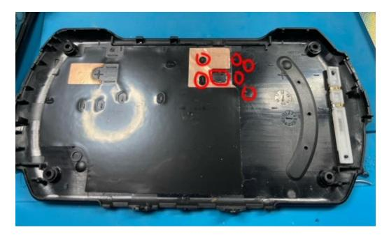
Additionally, you will want to cut flush the small plastics in the highlight area below. This will help reduce any bulging caused by the SD memory card reader.
