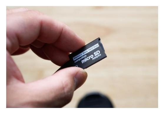
4. Open the M2 slot cover on the PSP Go and Insert the adapter in. Once you slot it in, you should hear a clicking sound which means the adapter is inserted and the system should be reading it. If you don't hear a clicking sound, make sure you're pushing it in all the way until it clicks.
