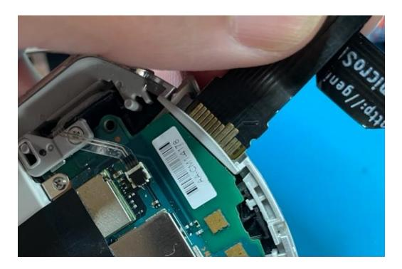
5. The adapter cable should easily slot into the back of your PSP Go, so now just place a piece of heat resistant tape or black tape (either are recommended) to hold the Memory Stick PRO Duo card and another piece to hold down the right and left side of the adapter cable as shown.
