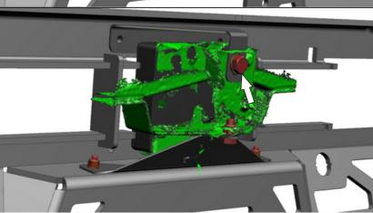
31. Fix the bottom part of radar using bracket  $N^2$ 1 (14), bolt M10x20 (C), washers 10 (P) and nuts M10 (L), as shown.
