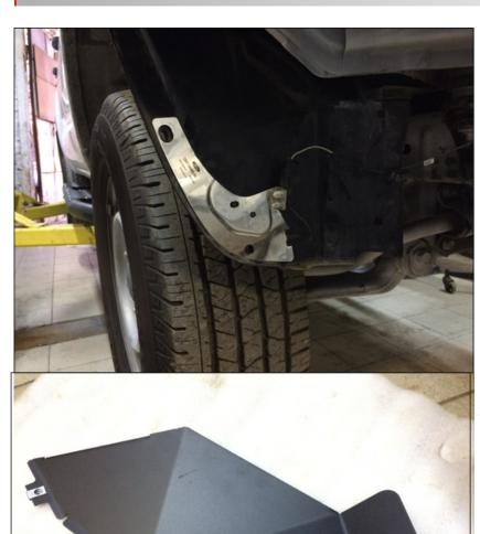
41. From right side, unstick antenna from the fender. Move antenna upper under the bar.
