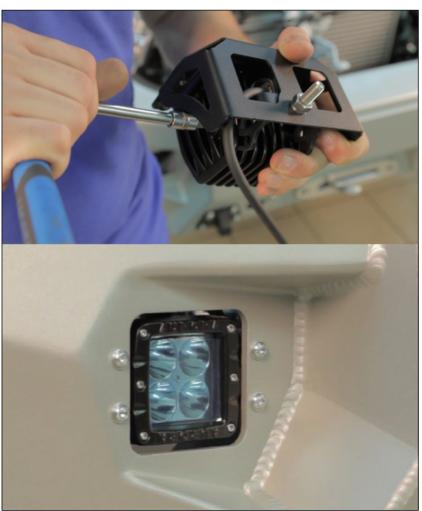
35. \* Mount LED lights into brackets (3). Tighten the joints.
