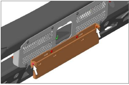
34. Adjust the angle of license plate. Tighten all connectors after that.
