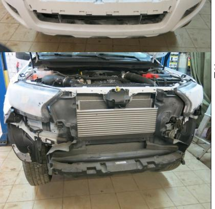
10. Remove the bumper by pulling the bumper towards you holding the sides.
