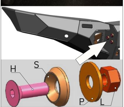
38. Place screw M10x30 (H) with countersunk washers (S) from both left and right sides as shown on the picture and secure with nuts M10 (L) and washers 10 (P).
