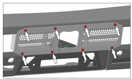
32. Install decorative pad (13), using screws M6x25 (G), washers 6 (M), nuts M6 (J), as shown.
