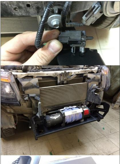
25. Fix temperature sensor to the bracket.
