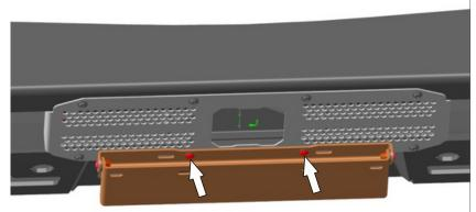
33. Install license plate (4) using screws M6x25 (G), nuts M6 (J) and washers 6 (M).
