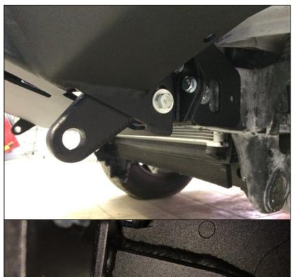
37. Install bumper body (1) onto the winch bracket (2). Fix its lower part to brackets using bolts M10x30 (D), insert nuts M10 (T) and washers 10 (P).
