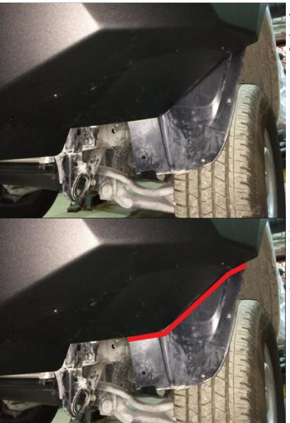
43. Install flaps (7, 8) using screw M6x20 (F) and washers 6 (M). Make sure the flaps are fixed inside of the bumper, not outside.
