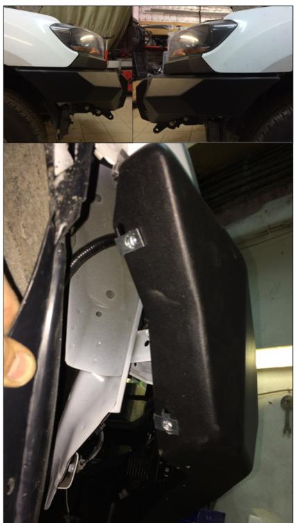
39. Adjust bumper until you have an equal gap between vehicle body and the bumper on both sides. Tighten bolts after that.
