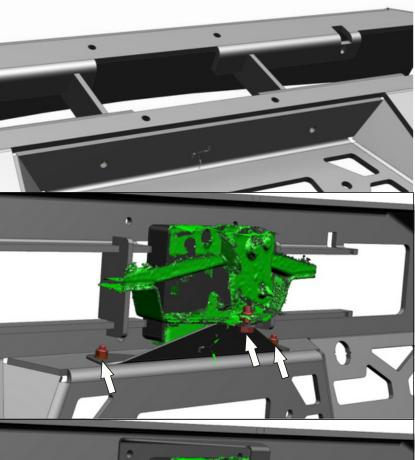
29.Cut the hole in bumper out, by follow the marked line Drill 6 pricked holes up to 8 mm
