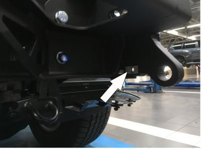
Install insert sleeves M10 (U) into the winch bracket.
