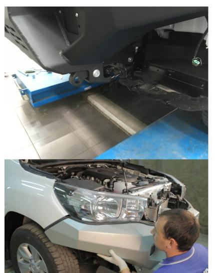
21. Insert screws M10x30 (E) with countersunk washers (O) in specified places on the left and right. Fasten to insert sleeves M10 (U).
