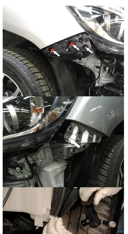
12. Remove pop rivets and screw out bolt M6. Dismount plastic fasteners of the bumper on splashboards on the left and right.
