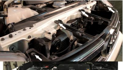
2. Screw out the screws which fix the radiator grill. Dismount the radiator grill by bending off plastic fixtures in the point of joint thereof with the bumper.
