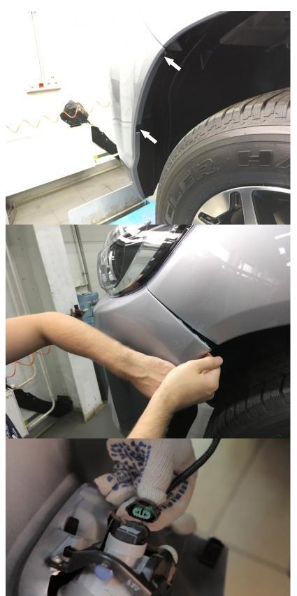
5. Remove the pop rivets under the wheel arch (3 rivets from each side).
