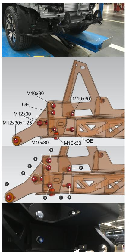
16. Install the winch bracket (2). Fasten with bolts M10x30 (A), washers 10 (J) and nuts M10 (H). Align the winch pad in vertical and horizontal planes.
