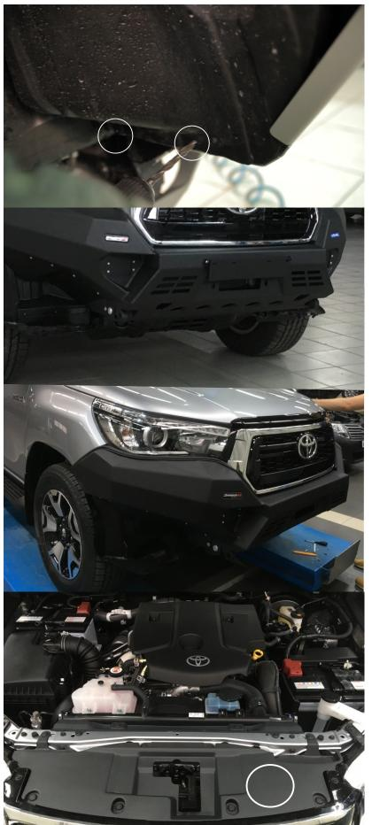
29. From the inner side of the arch, mark two holes in plastic wing flaps opposite to holes in aprons (7, 8). Drill hole dia. 6 – 8 mm. Through the obtained holes, fasten aprons (7, 8) with screws M6x20 (F) with penny washers 6 (L).
