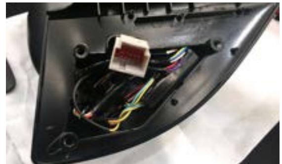
Remove gasket to reveal wiring.
