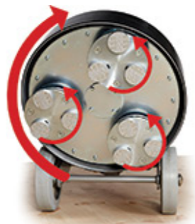
Figure 4-1 Illustrates the rotation of the grinding heads versus the gear barrel.
