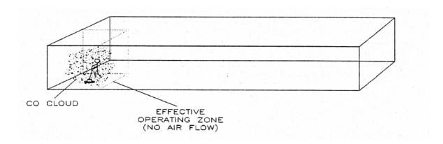
Stripping is quite a different type of operation than burnishing, and carries with it substantially more hazards, as stripping is a low movement operation compared to burnishing (less floor space for the same time). As shown in Model 1, the CO concentrations rise quicker as the "Effective Operating Zone" is a small area compared to the total building size.
