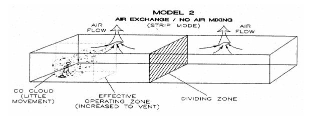
Notice the CO concentration and the Effective Operating Zone with air exchange. The CO cloud is still concentrated in a small area. Note the "Dividing Zone" shown above, this is the line where airflow changes direction. In Model 2, air changes are cut in 1/2 as little or no CO crosses the Dividing Zone to be exhausted.
