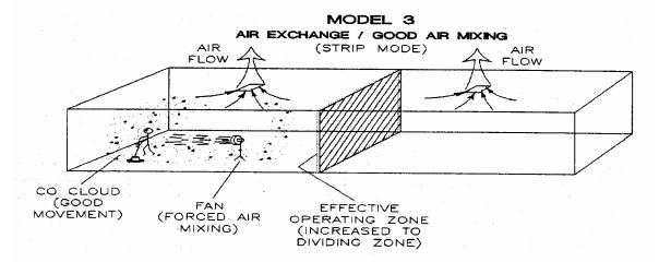
Notice the CO concentration and the Effective Operating Zone (Expanded to the Dividing zone) with air exchange and forced air mixing. The CO cloud is still concentrated on one side of the Dividing zone. Note the "Dividing Zone" shown above, this is the line where airflow changes direction. In Model 3, air changes are cut in 1/2 as little or no CO crosses the Dividing Zone to be exhausted.
