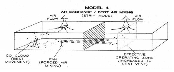
Notice the CO concentration and the Effective Operating Zone (Expanded through the Dividing zone to the second vent) with air exchange and forced air mixing through the dividing Zone. The CO cloud is diluted with the available air in the building. Note the "Dividing Zone" shown above, this is the line where airflow changes direction. In Model 4, air changes are full as forced air mixing has moved and mixed the CO between all air zones.
