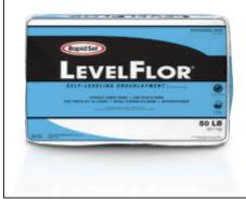
**CURING:** No curing is required under moderate conditions of 70°F (21°C). If used in exterior applications, apply a fine water mist to the newly hardened surface of Rapid Set® LEVELFLOR as soon as it can be done without marring the surface and continue until one hour after final set. Avoid excessively dry, windy, hot or sunny conditions.
