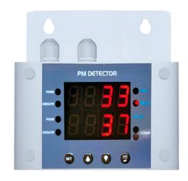
Utilizing a laser and optical sensor, the PM sensor measures light scattered from particles passing through the laser beam. The optical sensor transforms this scattered light into electrical signals, which are then processed to yield mass measurements of PM1, PM2.5, and PM10. The PM Detector's 2-line display allows simultaneous monitoring of PM2.5 and PM10, or it can be configured to display PM1 and PM10 together as per field requirements.
