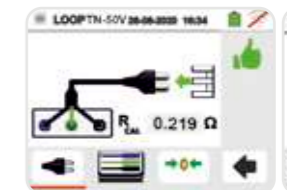
Zero-loop: compensation of the resistance of the test cables used for Loop impedance measurement.
