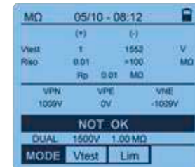
DUAL insulation verification with direct outcome: NOT OK
