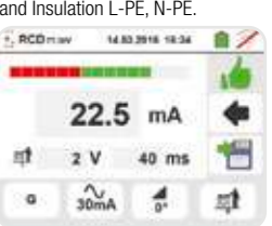
Result of ramp test on RCD.
