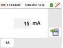
Measurement of leakage current with optional clamp HT96U.
