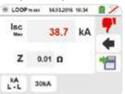
Negative result of breaking capacity test.
