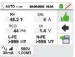
Autosequence: automatic sequence of measurements of Overall earth resistance, RCD test and Insulation L-PE, N-PE.
