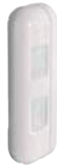
01739 Passive infrared presence detector for the protection of building exteriors, 12-metre curtain-effect detection on each side (left and right), PET immune, IP55, 1 input for acoustic control, 2 NO and NC 28 Vdc 0.2 A relay outputs, surface mounting, 10-28 Vdc 38 mA power supply
