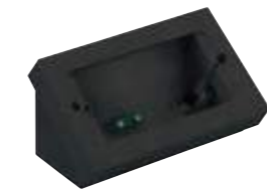
▲30784.G Tilted table mounting box, with variable height, for the installation of 4 modules. In the lowered version, connector blocks with a maximum depth of 32 mm can be installed; if you turn the cover the maximum depth extends to 44 mm. The socket outlet with USB, 30210. USB, cannot be installed. To be completed with mounting frame and cover plate.
