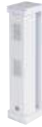
01740 Curtain-effect detector to protect entrances and openings such as doors, windows, covered terraces, corridors and French doors, short-range curtain-effect detection with adjustable lens up to 2 m or 5 m, PET immune, anti-masking function, 1 NO or NC 28 Vdc 0.1A relay output, surface mounting, 9.5-18 Vdc 20 mA power supply
