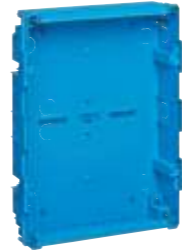
V53324 24-module flush mounting box (GW 650 °C) for masonry walls. Dim. 316x423x80 mm
