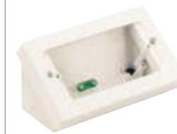
▲30784.B Tilted table mounting box, with variable height, for the installation of 4 modules. In the lowered version, connector blocks with a maximum depth of 32 mm can be installed; if you turn the cover the maximum depth extends to 44 mm. The socket outlet with USB, 30210. USB, cannot be installed. To be completed with mounting frame and cover plate.
