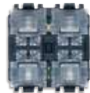
▲30484 4-button with 1 + 1 W RMS stereo amplifier, 2 x 8 Ω speaker outputs, RGB LED location in darkness with brightness control, to be completed with interchangeable half-buttons - 2 modules. Depth: 37,2 mm
