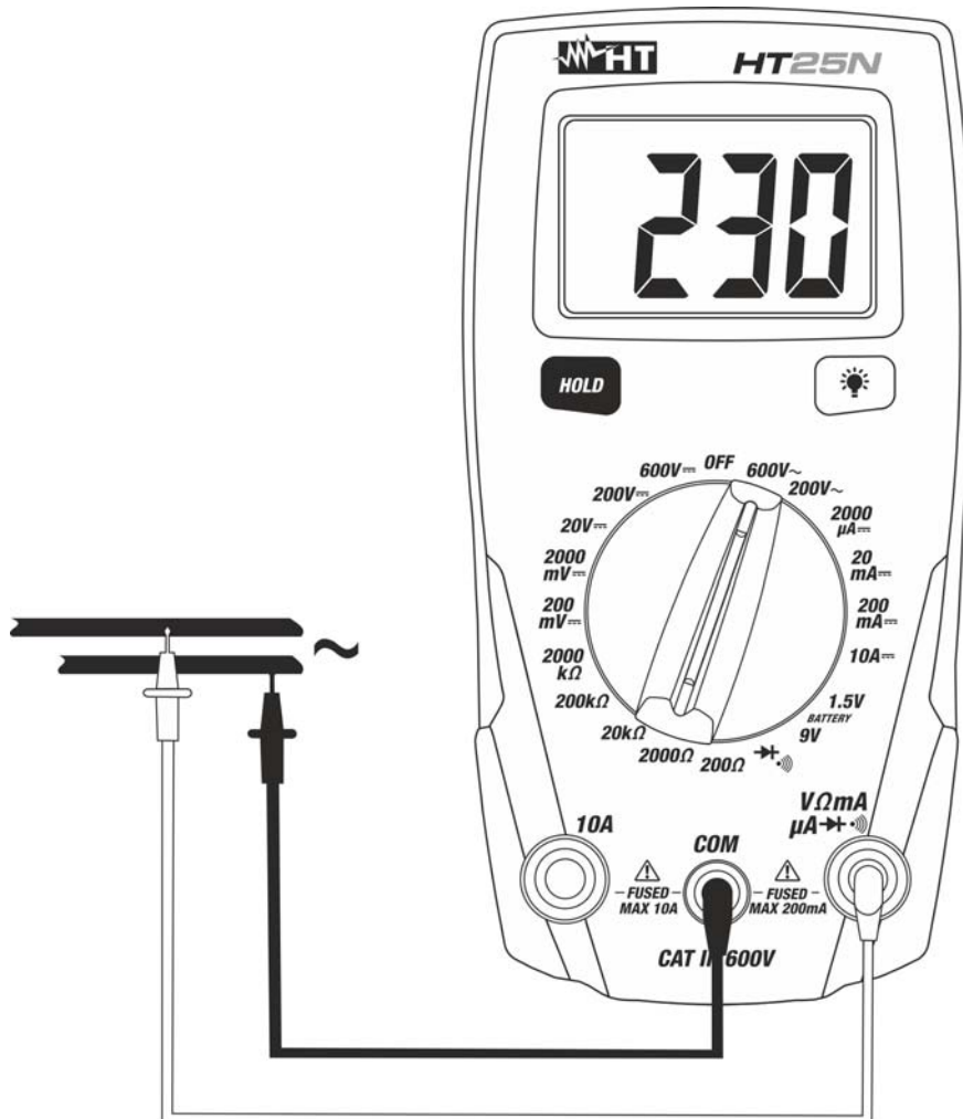
Fig. 3: Using the instrument for AC Voltage measurement
