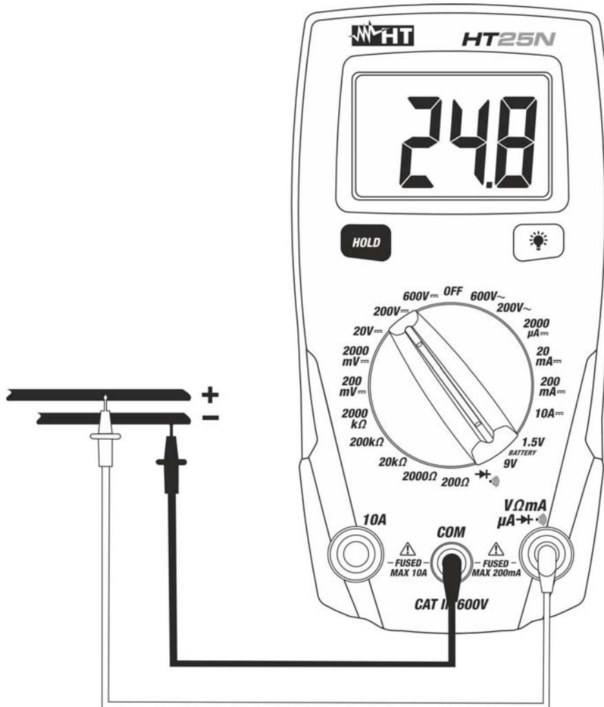
Fig. 2: Using the meter for DC Voltage measurement
