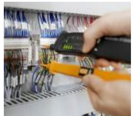
Troubleshooting with bipolar voltage tester incl. measurement probe according to IEC 61243-3
