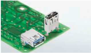
Webcode # 11420 USB 3.0/2.0 solder connection (THT) PCB jack for wave soldering process
