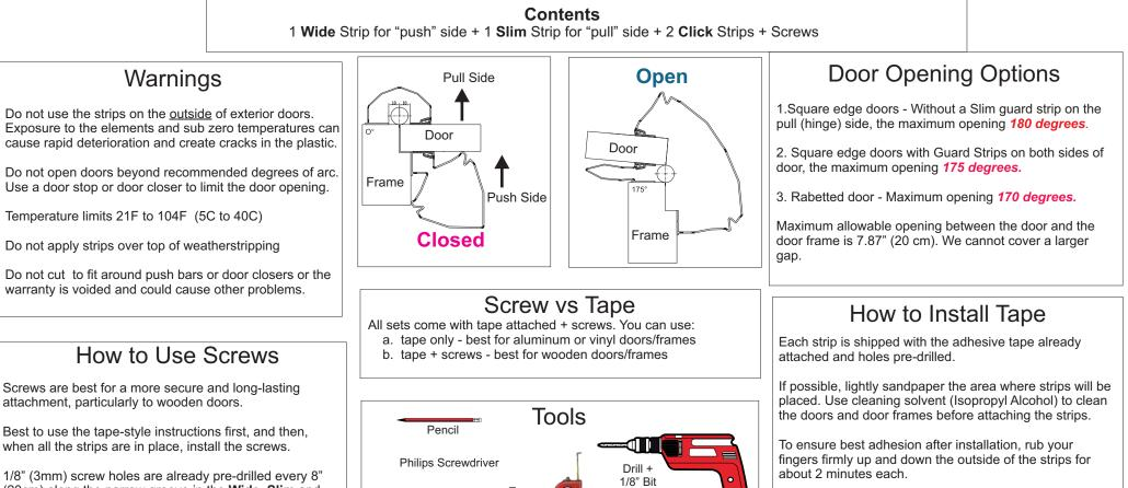
1/8" (3mm) screw holes are already pre-drilled every 8" (20cm) along the narrow groove in the Wide, Slim and **Click** strips. Bottom screw to be not more than 1 ½" from the floor to reduce peeling. Drill extra holes as needed.
