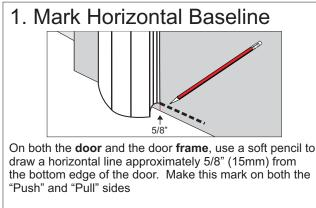
The purpose is to mark lowest point to install guard strips.
