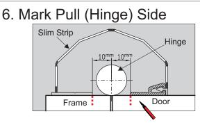
On each side of the "closed" door, draw a vertical line 0.4" (10mm) from the center of hinge. Make this vertical line on both the door and the door frame.
