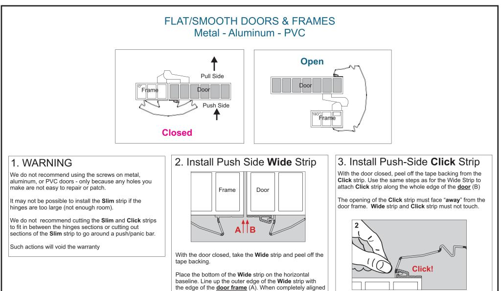
the edge of the door frame (A). When completely aligned with the whole frame, press the top part of the Wide strip into place. The other half of the Wide strip is still loose at this point.
