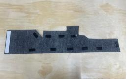
**Back Wall:** Remove the "loop" side of the hook & loop and discard. The hook is strong enough to hold the factory Polaris mat on the back wall. If you have issues reinstalling your bolts through the back wall don't use the big washers that were on them.
