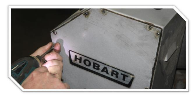
**3:** Remove the mounting bolts from the VFD and support the VFD outside of the electrical cabinet.
