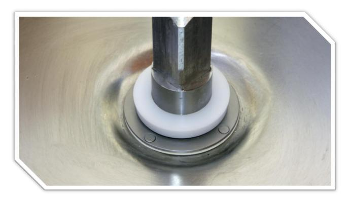
24: Fill the bowl with enough water to cover the seal and check for leaks.
