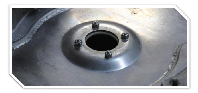
**15:** Remove any old silicone / RTV from the upper support bracket on the electrical cabinet.
