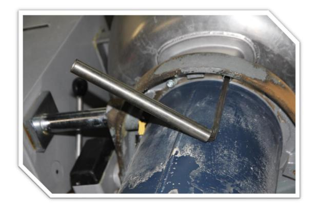
**8:** Tilt the machine vertical. Remove the upper bowl support from the electrical cabinet. You will have to break the seal of the OEM silicone sealant.
