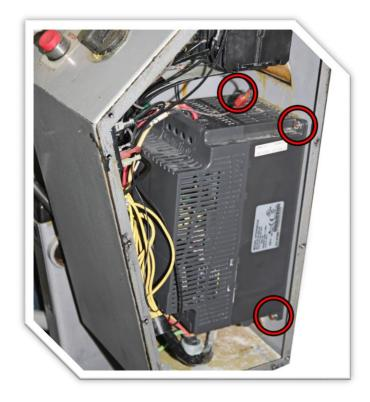
**4:** Unbolt the upper bowl support bracket from the inside of the electrical cabinet. This will also unbolt the handle shaft assembly, remove and set aside.
