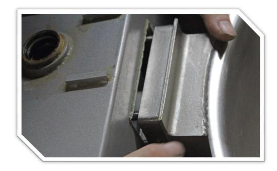
**9:** Remove the bowl. Install the drill jig from the inside of the bowl using the bolt, nut and washer.
