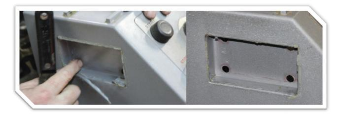
**16:** Apply food grade silicone / RTV to the upper support bracket. Apply liberally and remove excess after installation.
