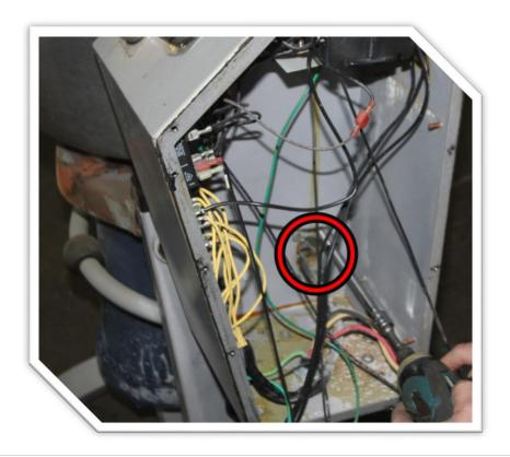
7: Carefully tilt the machine horizontal and remove the 4 bowl mounting screws. A cheater bar is recommended as the short side of the allen keys will not reach.
