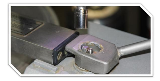
**6:** Locate the nuts for the lower support bracket. Only remove the top two bolts and unscrew the bottom two 50% of the way. This will allow the electrical cabinet to pivot out of the way enough for the bowl to be removed. Avoid pinching the motor leads as the cabinet pivots. It is best to have someone else hold the cabinet in place when the bowl is removed in the next steps.
