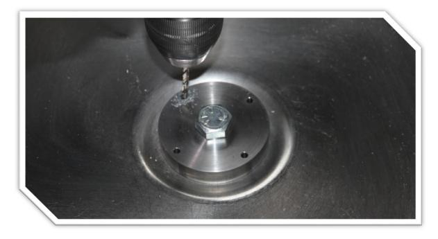
11: Remove the drill jig from the bowl and use a flat file to clean up any burrs on the bottom of the bowl. Check and clear any burrs on the inside of the bowl.
