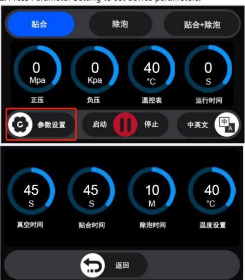
3. The factory default parameters are temperature: 40°C, vacuum time: 45 seconds, bonding time: 45 seconds, and defoaming time: 10 minutes.
