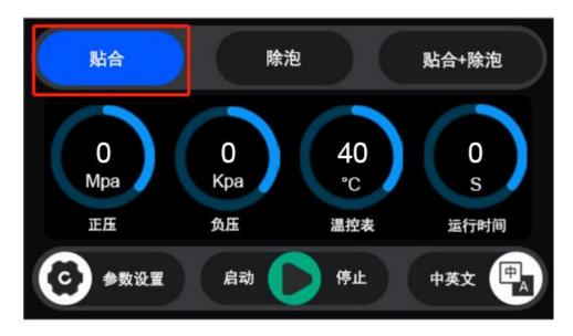
Press the start button, the device can start to work, the machine starts to vacuumize, runs to the set bonding time, the pressure jumps, at this time the device starts to bond, when the set bonding time is reached, the device starts to deflate, and the negative pressure value returns to zero , the fit is complete
