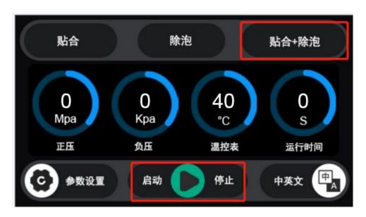
4. After starting, note that the negative pressure value on the display screen continues to rise, which means normal. If the pressure value does not rise after starting, please contact after-sales technicians to solve it for you.
