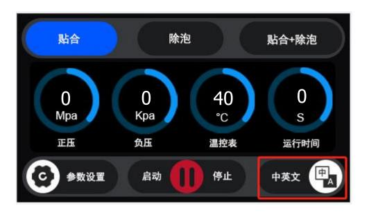
2. Press Parameter Setting to set device parameters.
