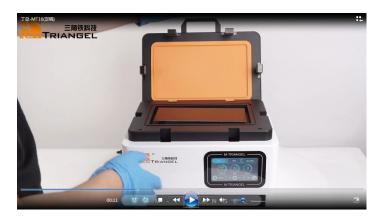
\*The placement of the screen is very important, which directly affects the final yield. The edge of the display window of the screen should be aligned with the edge of the sponge pad, so as to completely avoid the cable. Pressure leads to waste screen. (If you have other questions that you don't understand, you can contact the aftersales technicians to answer for you.)
