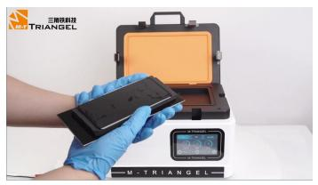
\*Note that after the cover and the LCD are closed, do not squeeze or press. Usually there will be a hollow in the middle of the bottom of the mold. Just press and hold the middle of the cover with your fingers, and then tap the LCD in the middle of the bottom of the mold to make the middle stick That's right, this is extremely important!
