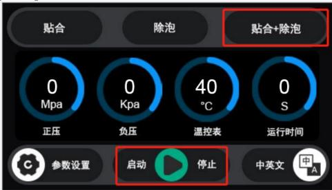
4. After starting, note that the negative pressure value on the display screen continues to rise, which means normal. If the pressure value does not rise after starting, please contact after-sales technicians to solve it for you.
