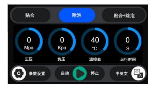
Press the start button, the device can start working, the positive pressure reaches 0.6MPA, and it runs until the defoaming time is set. When the device starts defoaming, when the set defoaming time is reached, the device starts to deflate, the positive pressure value returns to zero, and the defoaming is completed.
