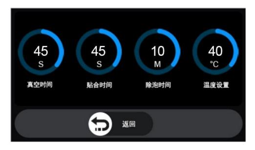
3. The factory default parameters are temperature: 40°C, vacuum time: 45 seconds, bonding time: 45 seconds, and defoaming time: 10 minutes.
