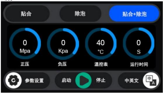
Press the start button, the device starts to work, observe the negative pressure gauge, temperature control gauge, and negative pressure gauge to zero, after the lamination is completed, the device automatically jumps to the
