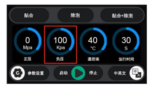
\* Different regions have different altitudes, which will affect the effect of vacuuming. The higher the altitude, the lower the peak value of negative pressure, and the best effect is when the negative pressure is above -88.
