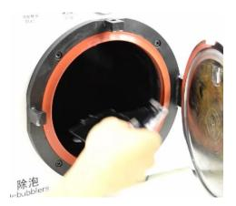
**Step 3:** Click start button to defoaming, and wait until it automatic release the air to finish defoaming. And then, open the door.
