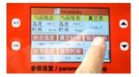
\* The air will be released by 30s vacuum time, and then the laminating plate will be slowly down with pressure 2-2.5kg. After
