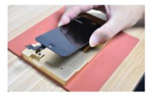
**Step 2:** Put the screen on the plate, and put them into the machine. Close the door.
