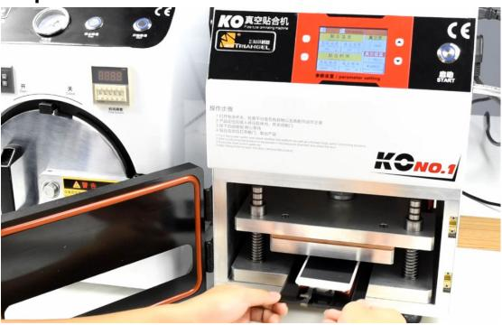
Open the laminating door, put the aligned screen into the machine.
