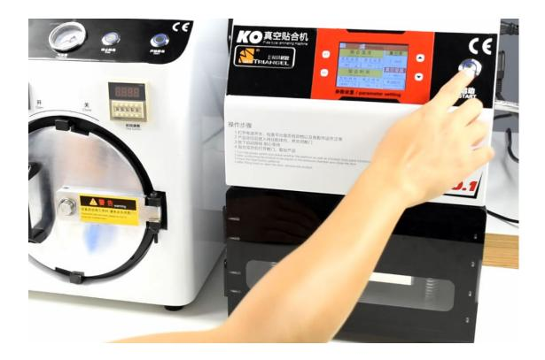
Open the door and click start button, the vacuum pump will automatically working. Pressing plate will auto-pressing after vacuumizing in prescribed time. After laminating, open the door.
