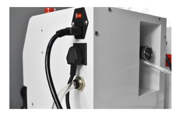
2) Insert the air compressor pipe to the pressure regulating valve interface back of the laminator.
