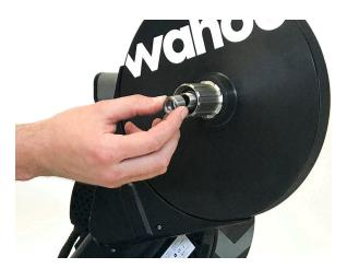
4. Remove the axle nut with a 17mm spanner. Set this nut aside (this will be needed later).
