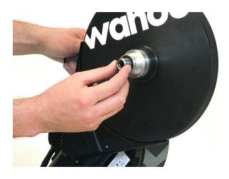
7. Screw the axle nut back onto the axle. Do it up finger tight; if it is too tight, it can damage the bearings in the adaptor.
