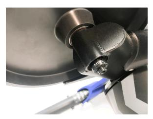
9. Slide the non-driveside axle spacer, with the135mm side facing out.
