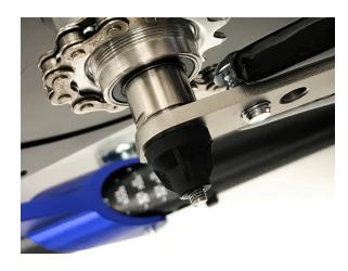
14. Tighten the axle screwer onto the dropout extension.
