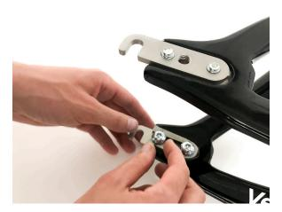
12. Bolt the dropout extensions to the outside of your frame with a 6mm Allen Key.
