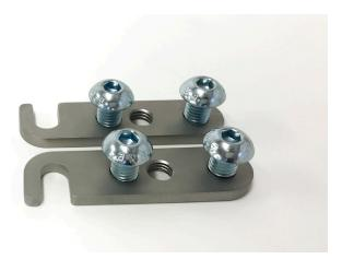
11. Screw two fastening bolts into a dropout extension.
