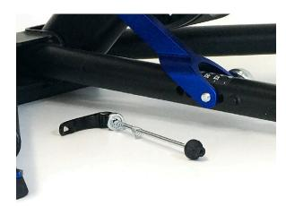
1. Remove the axle skewer and set aside (this will be needed later).
