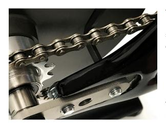
15. Adjust the chain tension by using a 8mm Allen Key to secure the front bolt in the dropout extension.
