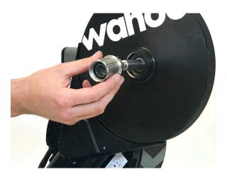
5. Slide off the free-hub body and the spacer behind it.
