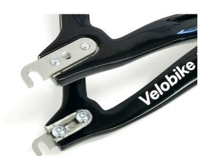
Note: Depending on where your dropout is for chain tension, there are two bolt holes to choose from.
