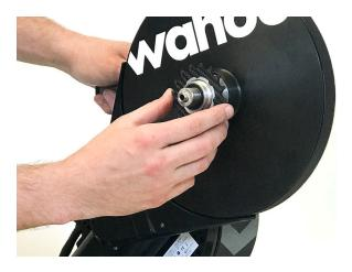
10. Screw on a fixed gear cog and lock ring.
