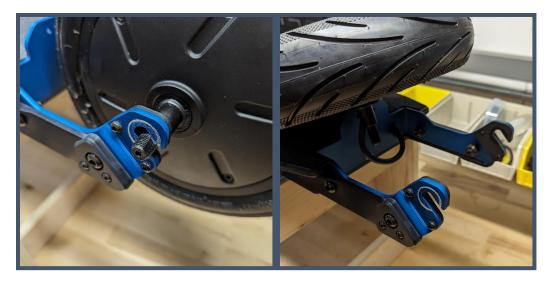
**Step 4.** Remove existing torque plates on each side and replace them with the new torque plates supplied with the rear fender. When installing these, it is recommended the screws be kept loose until the rear wheel is reinstalled.
