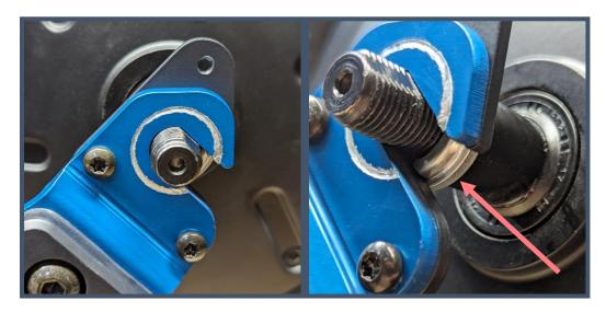
**Step 6.** Reinstall the rear wheel axle nuts. **CAUTION: The rear wheel axle must be pressed fully into the wheel carrier slot.** To ensure of this, use downward pressure on the rear of the deck with the rear wheel on the ground or table while tightening the nuts. The rear axle nuts can be torqued to 65 Nm.
