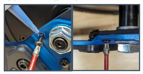
**Step 8.** Using a 2.5mm hex key, install the rear fender bracket onto the rear fender with the supplied M4 flange Screw. Do not use any thread locker on this screw. **NOTE: Match the orientation of the rear fender bracket as shown.**
