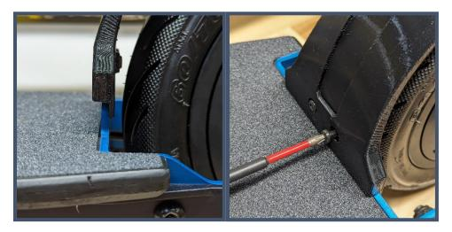
**Step 10.** Align the ends of the rear fender bracket to the outside of the torque plates as shown. Apply a small amount of thread locker to the ends of the two provided M4 x 6mm screws. Install the screws using the T20 Torx key. **NOTE: Do not add any more thread locker than necessary. The proper amount shown is approximately the size of a sesame seed.**
