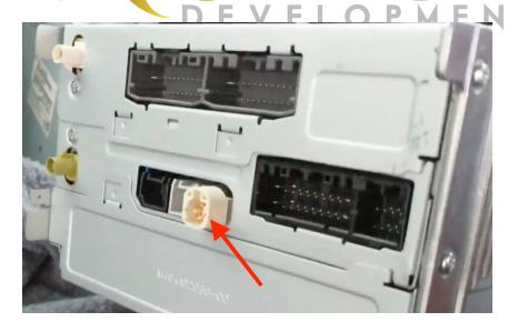
Once installed, to switch in/out of CarPlay display, long press highlighted button
