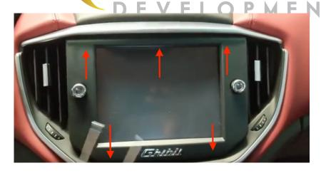
3) Remove 2 x cables from rear of the plastic trim, remove 4 screws holding in vent unit
