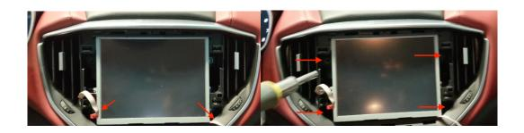
4) Remove electrical connectors retaining air vents
