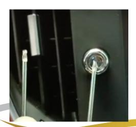
2) Use trim tool to carefully remove bezel (clip locations shown with red arrow - recommended to start from top clips
