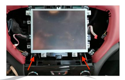
b) Plug inline connector behind headunit – power passthrough plugs in line behind matching factory power cable
