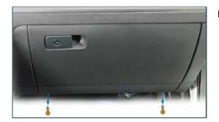
Remove screws from bottom of glovebox lid.
