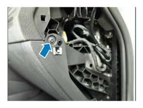
Remove marked screw from side panel as shown.
