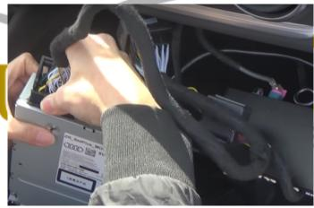
Connect quadlock connectors from CarPlay wiring in line between original connector and infotainment unit (see wiring diagram for clarification)
