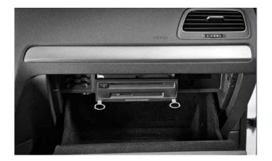
Open glovebox, see VW infotainment unit and insert the two release keys, push carefully until they engage and are held in the slot.
