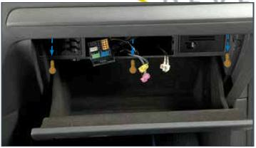
Remove screws from top lip of glovebox in marked locations.
