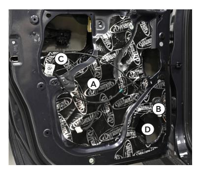
**Outer Door Patches** - Install on inside of outer door skin by passing through access holes in inner door structure. **Tip:** Partially pre-peeling release paper backing and folding aluminum faces together makes this easier. Adhere to door. Smooth with Dynamat roller for best results.
