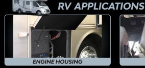
Use DynaCore to line the surfaces inside the enclosures of power generators and air compressors. They absorb heat and the sound waves of the enclosed area.
