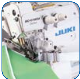
Rolling in tape - MO-6745DA-FF4-360/N077 (N077: Clean finish top and bottom)
