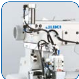
Presser lifter drive mechanism air cylinder. Thread trimmer drive mechanism air cylinder.
