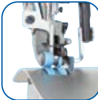
Alternating vertical movement mechanism
