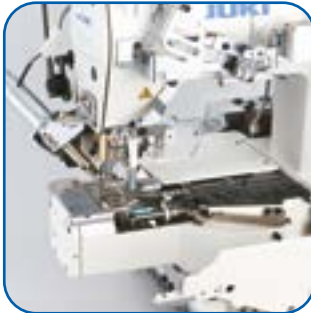
Electromagnetic needle thread / looper thread trimming device
