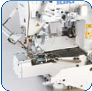
Electromagnetic needle thread / looper thread trimming device
