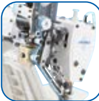
New type belt feed mechanism
