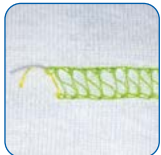
By making a knot at the end of sewing the thread won't be frayed.
