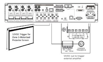
There are four 12Vdc trigger outputs which correspond to the four output zones. When a zone is powered ON by the RX 800 keypad, the corresponding zone sends 12Vdc to the trigger output jack. The triggers can be used to automatically switch peripheral equipment ON or OFF.
