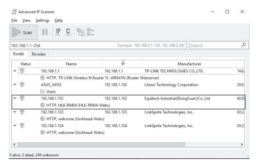
Then enter the IP address of RX 800 to the IE browser (shown as below), ensure the Serial Configure is 9600,n,8,1. After finishing this step, RX 800 could be controlled through the local Network.
