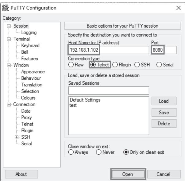
Click Telnet, enter the IP address of RX 800 and port: 8080.
