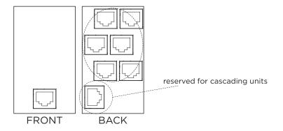
Connect the other end of the terminated Cat5e/6 to the RJ 45 port on the back of the assigned keypad and installation is complete. Complete zone and source control as well as IR and power are provided through the single Cat5e/6.
