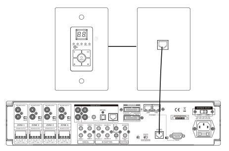
Without power being connected, connect a Cat5e/6 cable to the RJ45 port labeled KEYPADS on the back of the AMP We recommend terminating the Cat5e/6 using the 568B standard.
