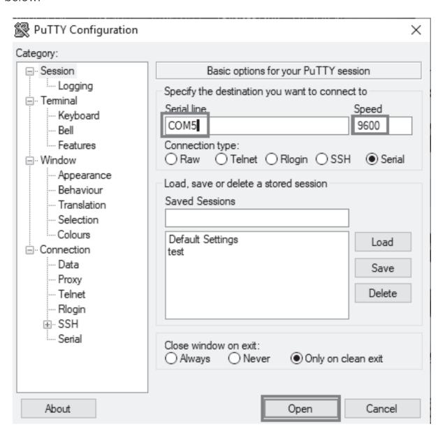
Click Serial, check the COM port and enter the Baud rate 9600. Click Open.
