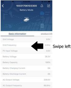
**[Basic Information]** displays basic information of the inverter, including AC voltage, AC frequency, PV input voltage, Battery voltage, Battery capacity, Charging current, Output voltage, Output frequency, Output apparent power, Output active power and Load percent. Please slide up to see more basic information.
